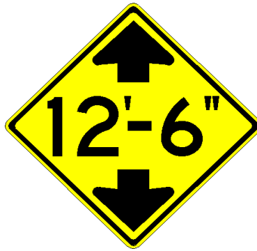
MUTCD Low Clearance (W12-2) Sign
