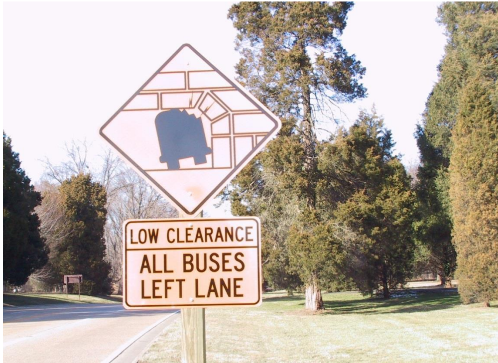
Photograph 7 – New low clearance sign developed by the National Park Service as a result of the Alexandria Avenue Bridge Overpass accident on November 14, 2004 in Alexandria, VA
