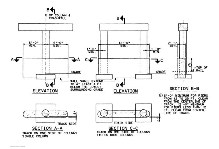
*Figure C-8-2-1. Pier Protection: Minimum Crash Wall Requirements (Not To Scale)*
