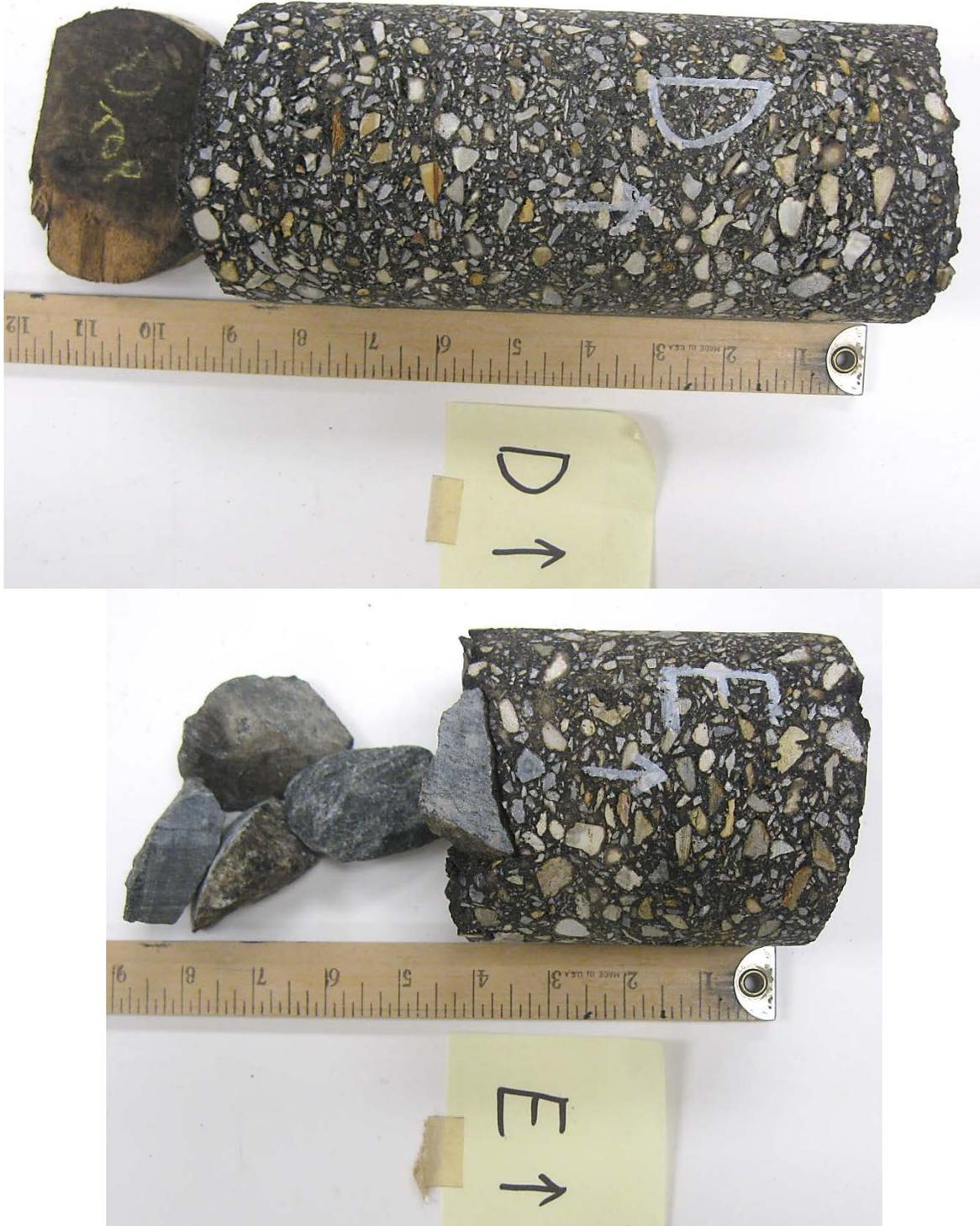
Figure 2. Photographs of cores D and E as-received for visual examination. Top end in each core placed to the right.
