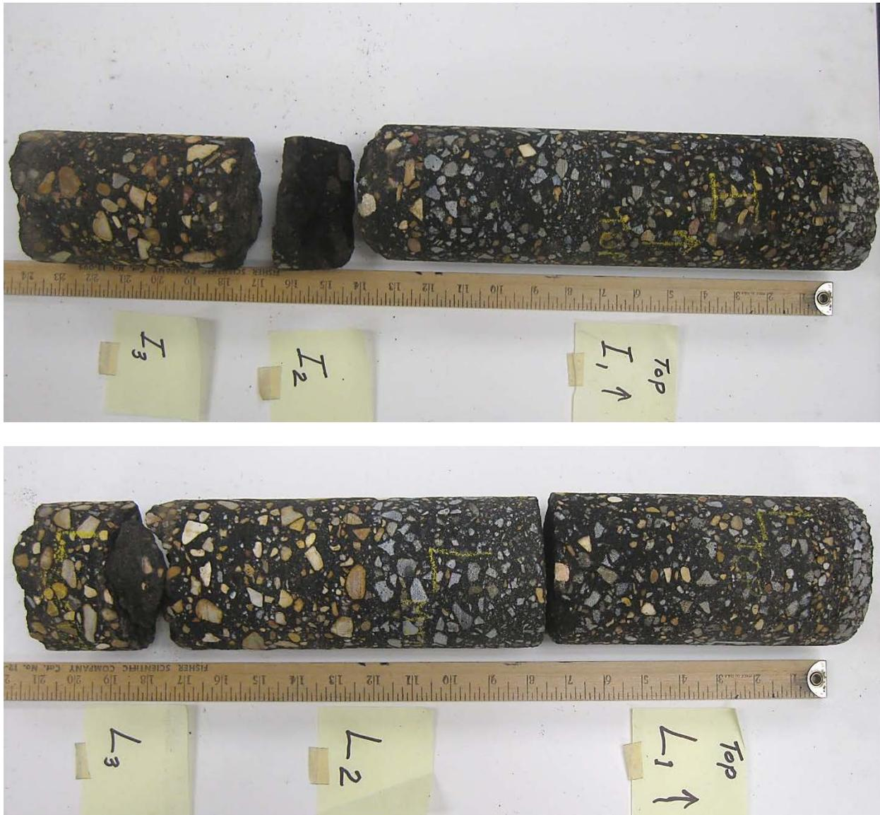
Figure 6. Photographs of cores I (eye) and L as-received for visual examination. Top end in each core placed to the right. Note that both cores received broken into three pieces.
