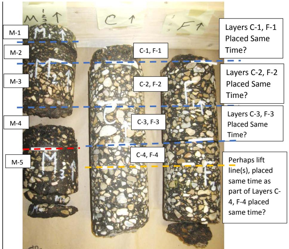
Figure 8 – Shows Biloxi NTSB Cores Away from the Rails; Cores L, I, M, C, and F lined up, with the core-tops up and with approximate layer lines and lift lines also shown.
