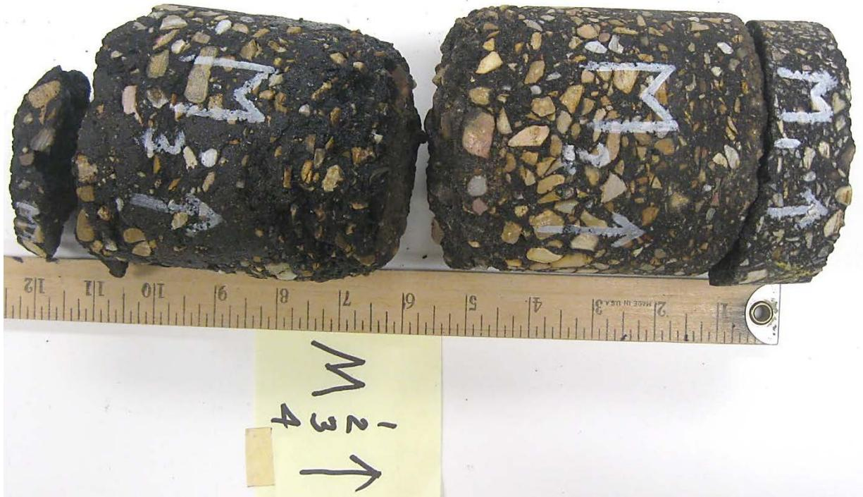
Figure 7. Photograph of core M as-received for visual examination. Top end placed to the right. Note the core was received broken into four pieces.
