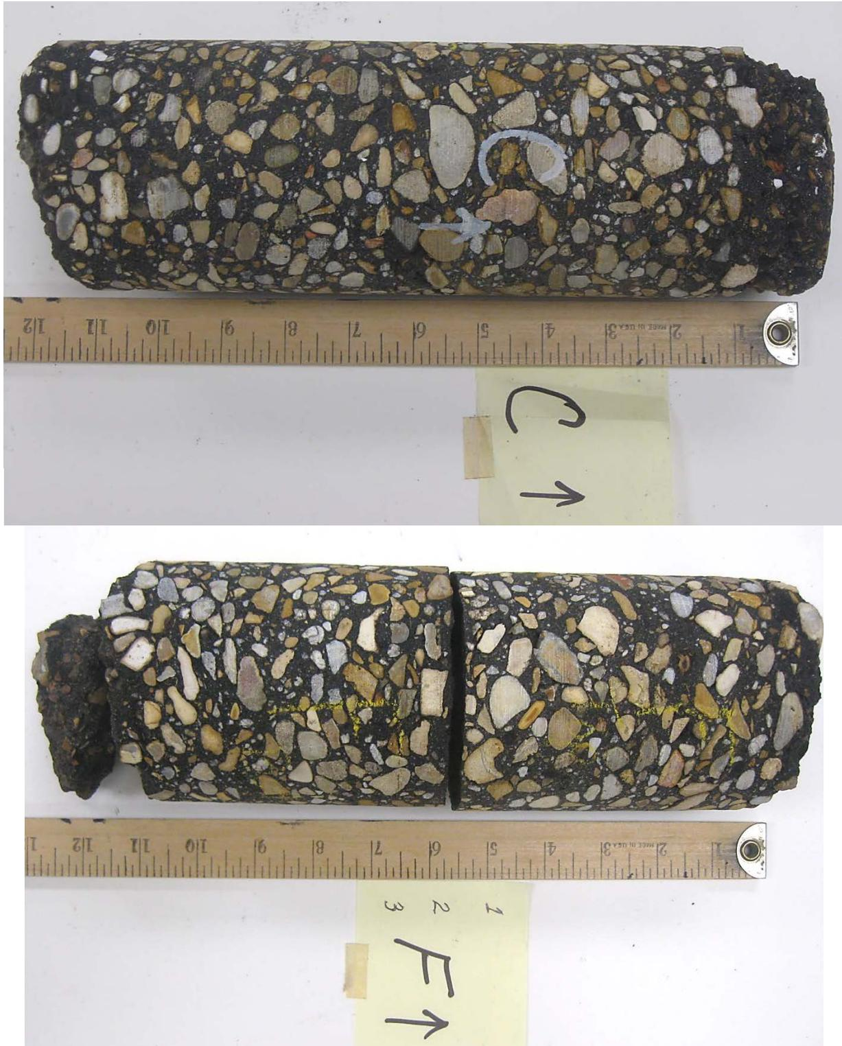
Figure 5. Photographs of cores C and F as-received for visual examination. Top end in each core placed to the right. Core 5 received broken in three pieces.
