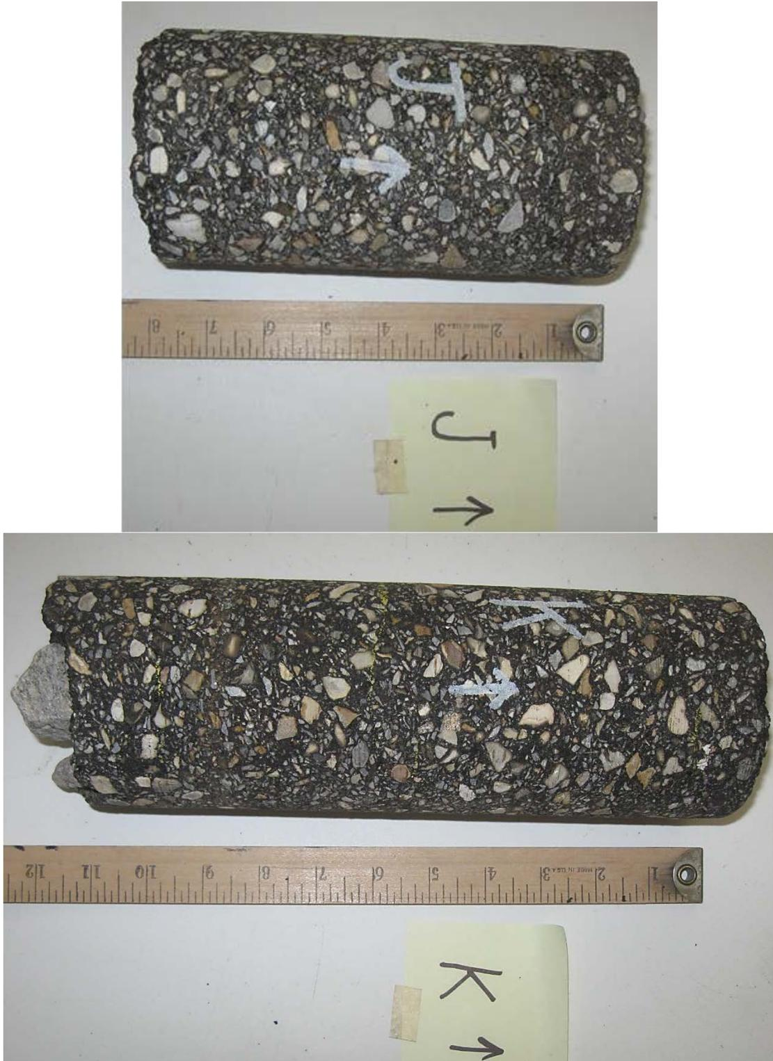
Figure 4. Photographs of cores J and K as-received for visual examination. Top end placed to the right. Note the crushed coarse aggregate ballast attached to the bottom end of the core K (left end).
