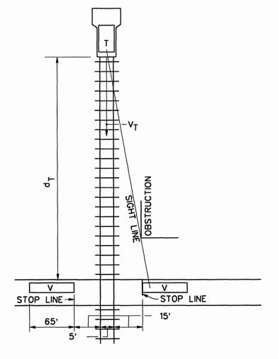
$d_{T}$  = sight distance along railroad tracks (feet)  $V_{T}$  = velocity of train (mph)
