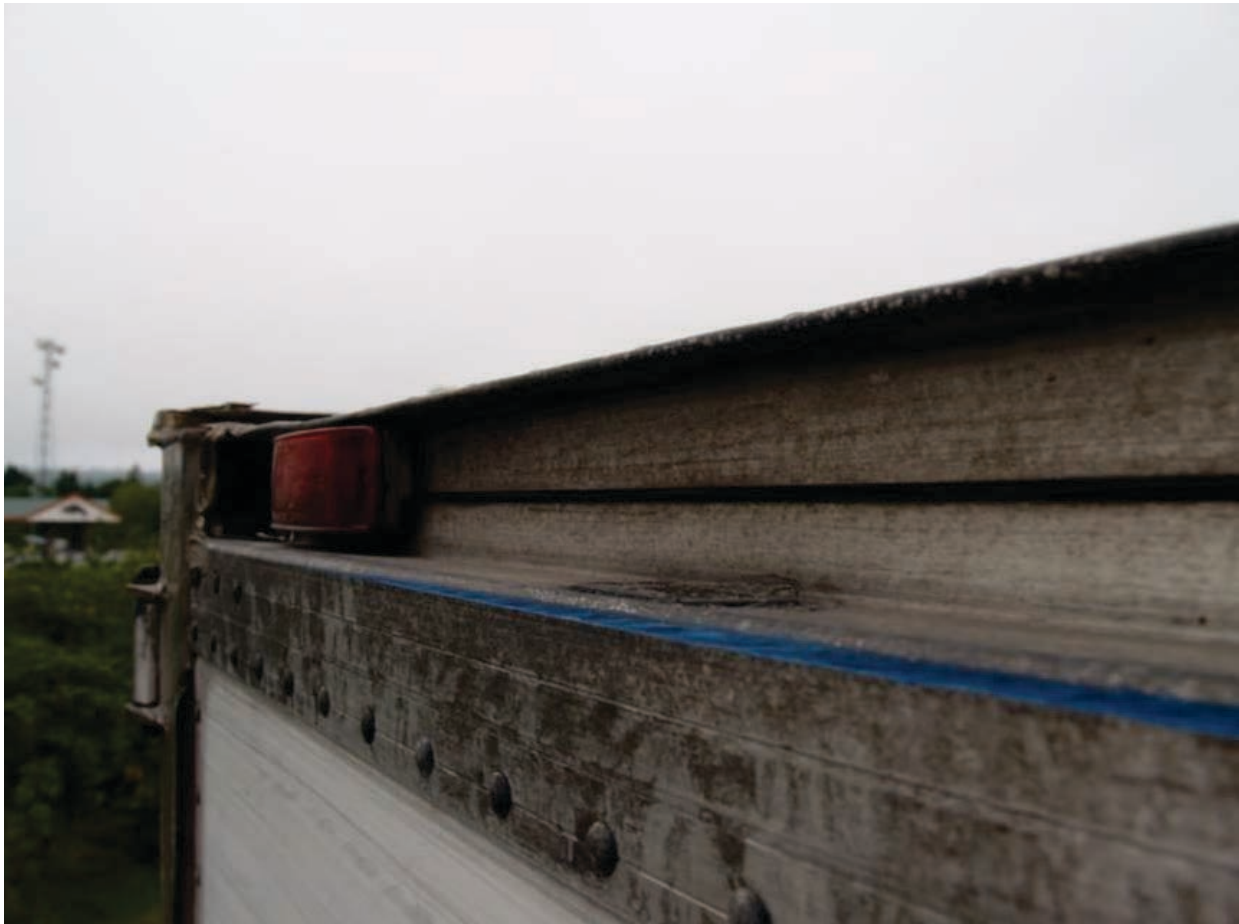
Figure 9. Blue transfer paint from the oversized load found postcrash on the upper right side of the refrigerated semitrailer of the 2000 Kenworth truck.
