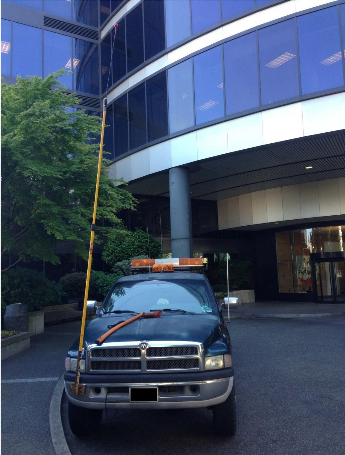
Figure 11. Pilot/escort vehicle, showing the placement of the height pole on the front bumper.
