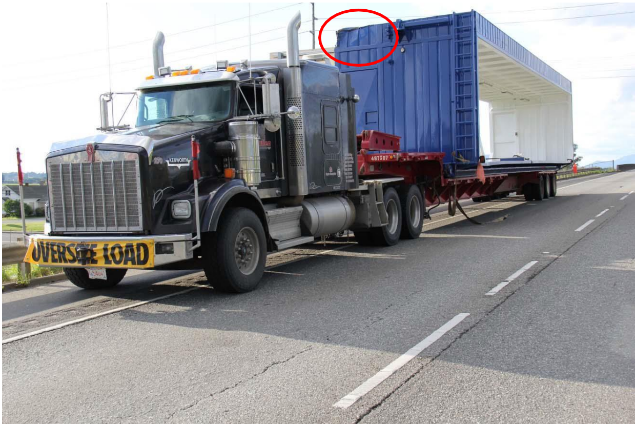
Figure 7. The oversize load, with the area of damage circled.
