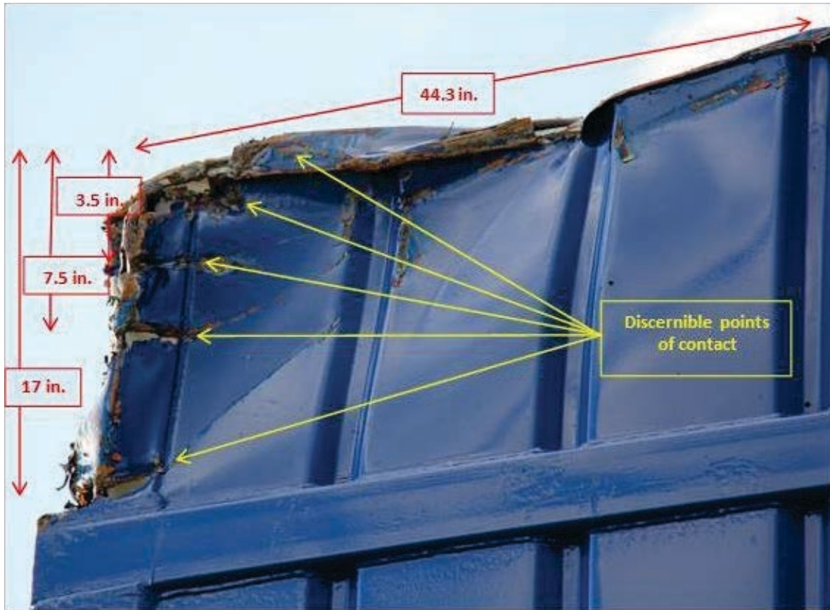
Figure 8. The upper right corner of the oversize load, with damage dimensions.
