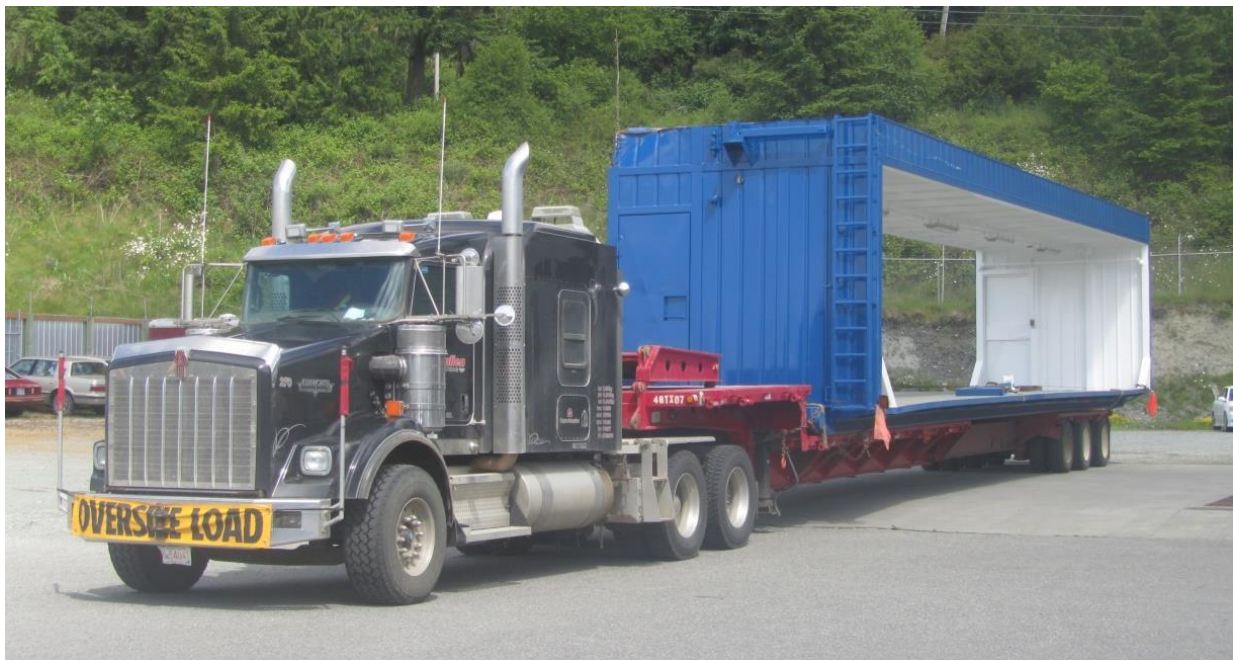
Figure 1. The oversize combination vehicle with the casing shed section loaded on it.
