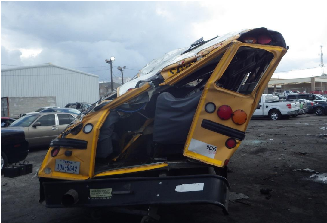
Figure 5. View of the rear of the HISD bus showing contact damage to the top left corner.
