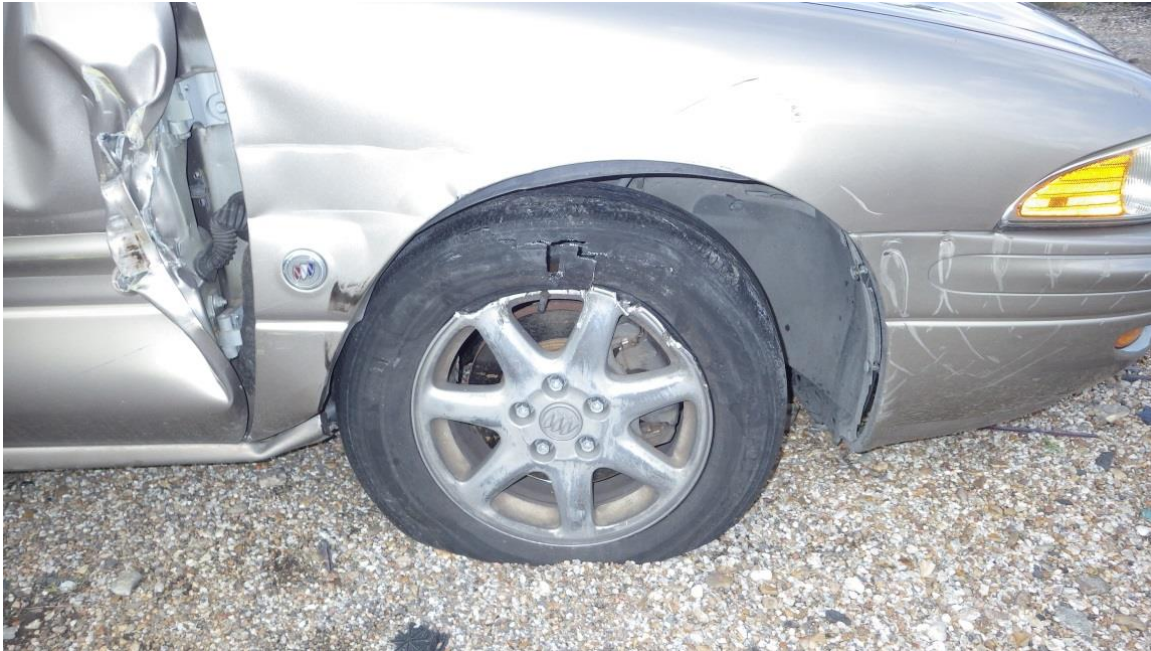
Figure 6. Pattern scratches and damage to the front right tire on the Buick LeSabre from contact with the HISD bus.
