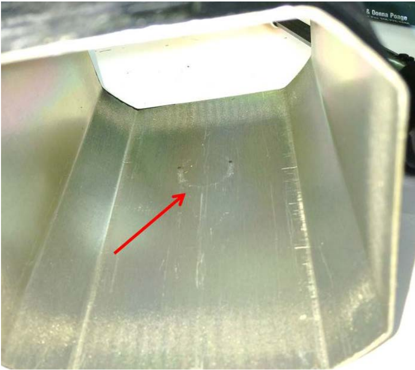
Photo 5 - Imprint left by lower pivot bearing on bottom of the case.
