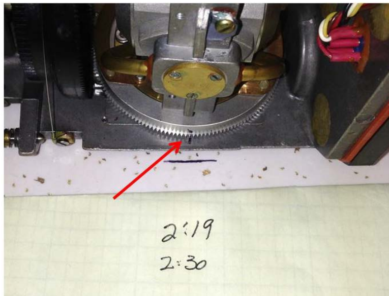
Photo 10 - Final alignment of spur gear and case index marks after the 11-minute test.
