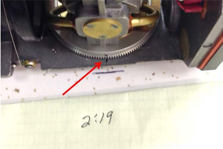
Photo 9 - Initial alignment of spur gear and case index marks.
