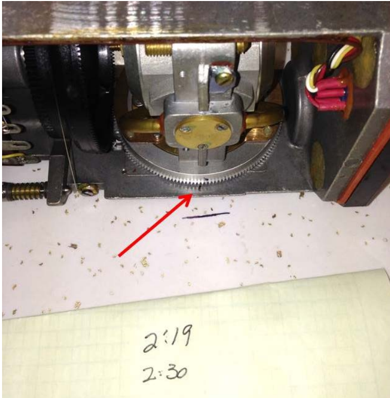
Photo 11 - Alignment of index marks after case was rotated slightly clockwise about the vertical axis.
