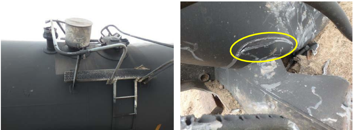
Figure 22: TILX 195386, top fittings (left) and A-end head pad separation (right circled), staging area, March 12, 2017.
