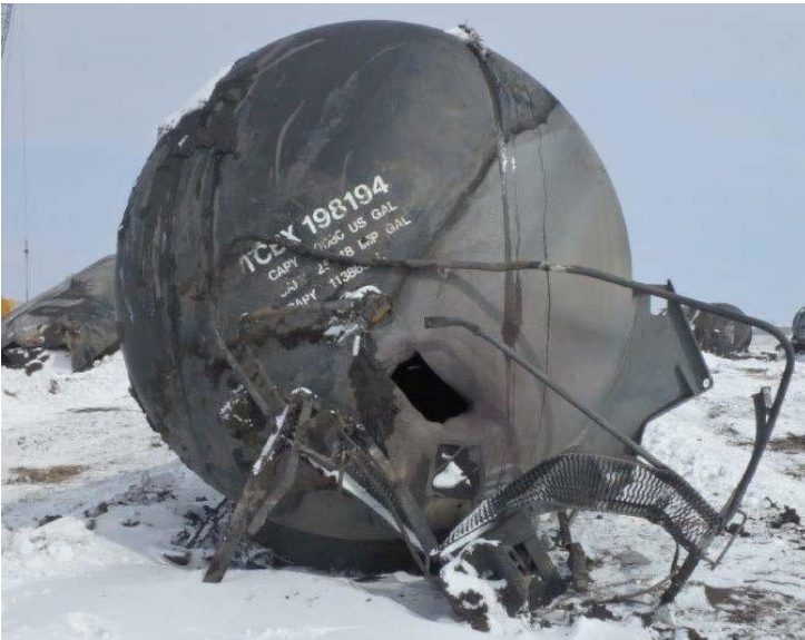
Figure 10: TCBX 198194, A-end head puncture, staging area, March 13, 2017.
