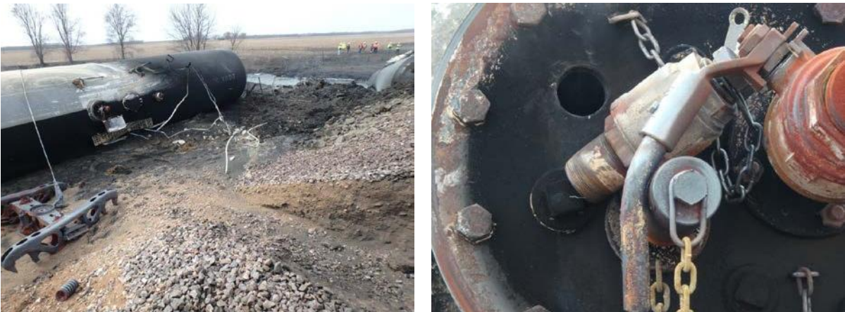
Figure 6: DBUX 301674, in-situ (left), multihousing flange with missing vapor valve (right), March 11, 2017.
