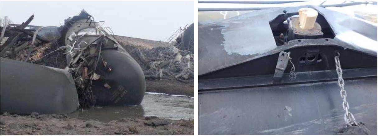
Figure 7: TAEX 2893, in situ (left), and in staging area (right) with plugged bottom outlet nozzle, March 11, 2017.
