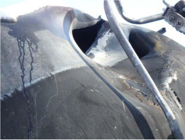
Figure 9: TILX 199147 A-end head puncture, March 11, 2017.
