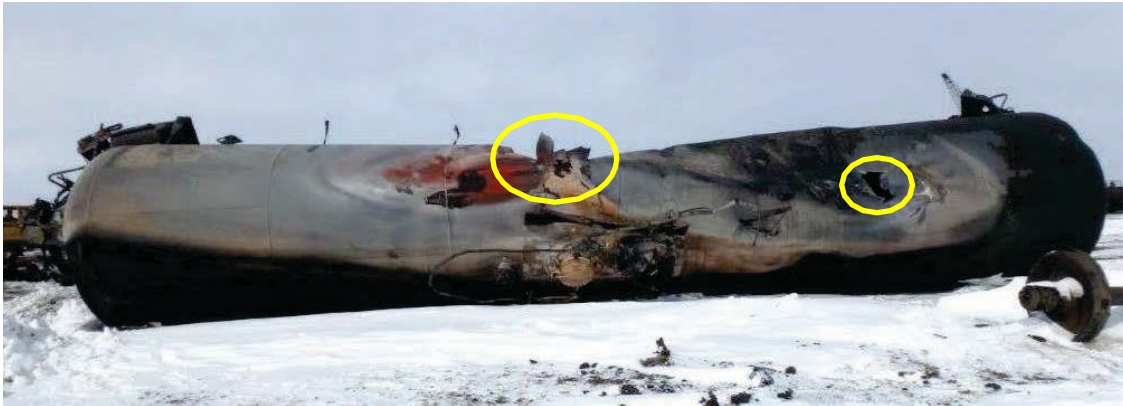
Figure 11: CTCX 732108 in staging area, breaching damage circled March 13, 2017.
