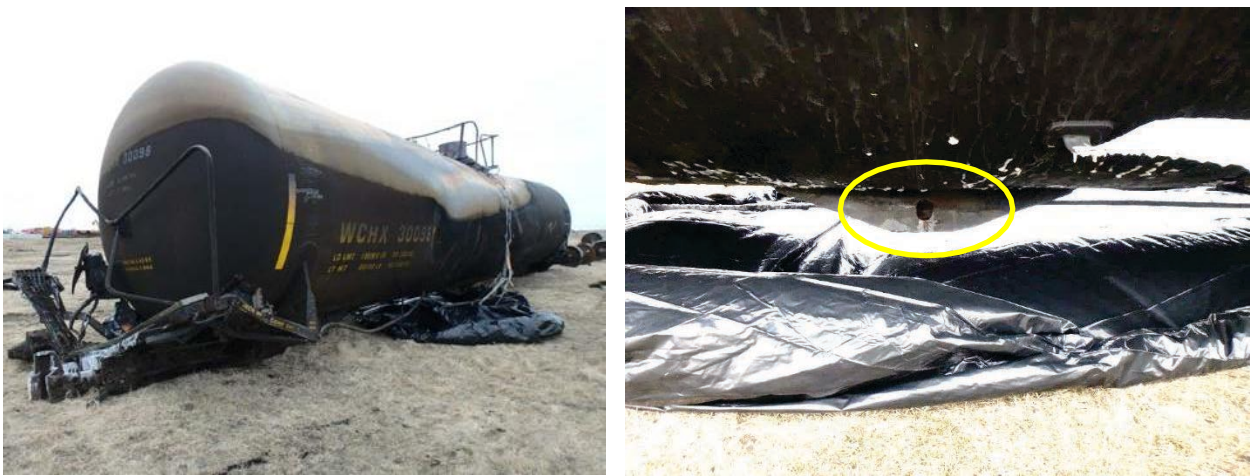
Figure 18: WCHX 30098 staging area (left), leaking bottom outlet (right), March 12, 2017.
