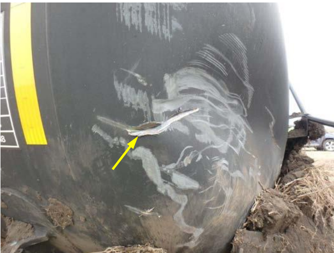
Figure 24: TILX 197615 gouge to A-end head (arrow), March 12, 2017.
