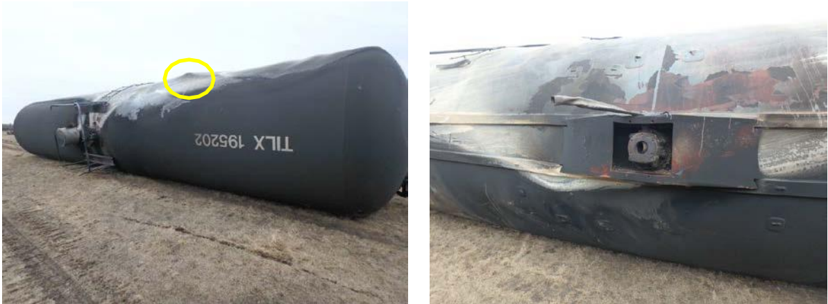
Figure 20: TLX 195202 Thermal tear (left circled) and open bottom outlet (right), staging area, March 12, 2017.
