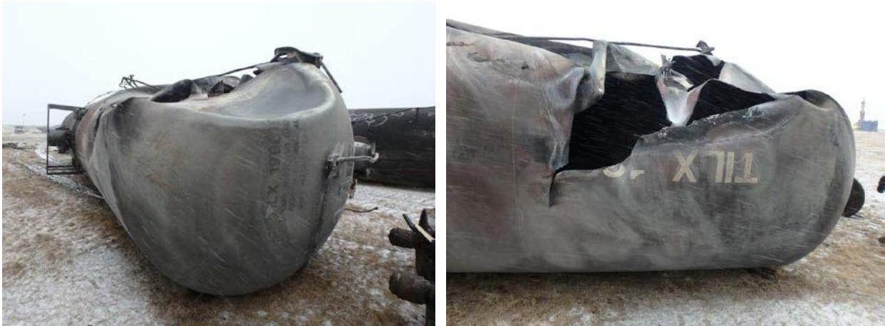
Figure 19: TILX 199819 A-end shell tear, staging area, March 12, 2017.
