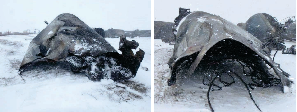
Figure 12: DBUX 302834, two halves of fractured tank car, staging area, March 12, 2017.
