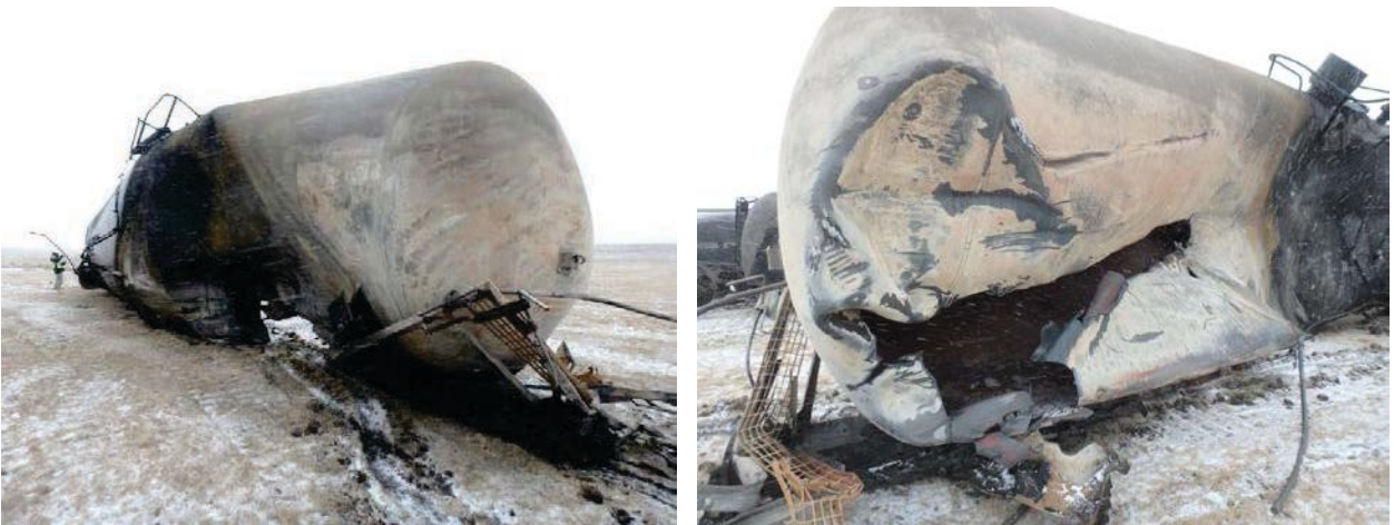
Figure 16: WCHX 30078 shell fracture (left) and head-shell tear (right), staging area, March 12, 2017.
