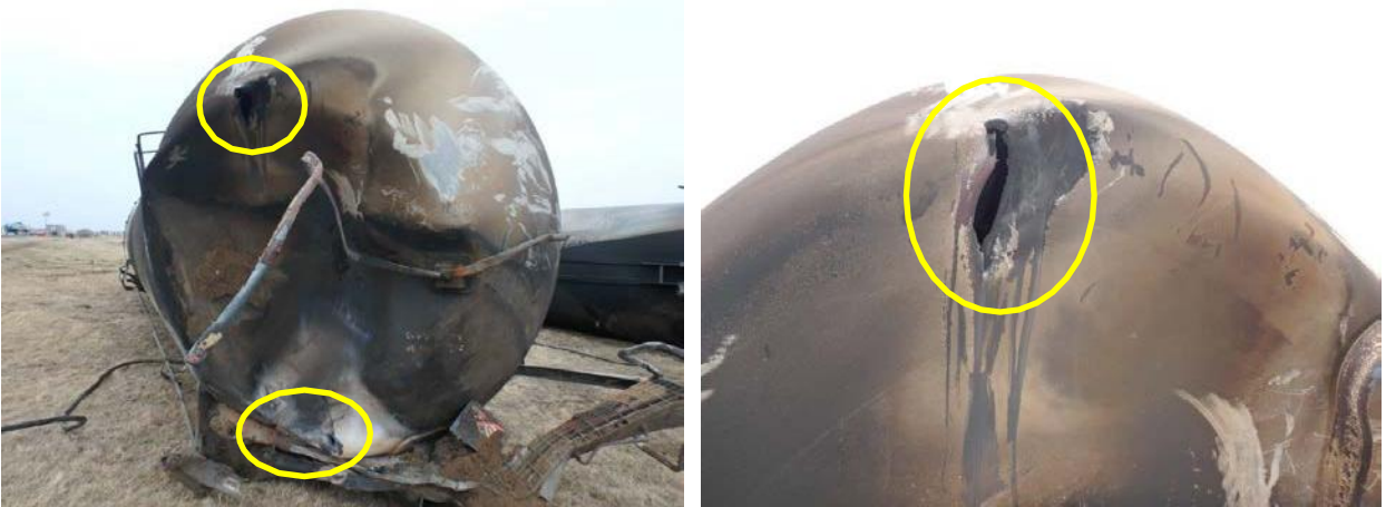
Figure 23: CTCX 731997 A-end head breaching damage (left and right circled), staging area, March 12, 2017.
