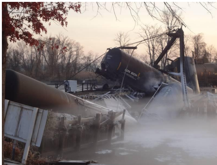
Figure 9 – View of derailed tank cars (at approximately 7:11 a.m. on November 30, 2012) in a fog or cloud with visible ice on the tank cars and in the water. 37 (Photograph courtesy of the wife of the Paulsboro Assistant Fire Chief)
