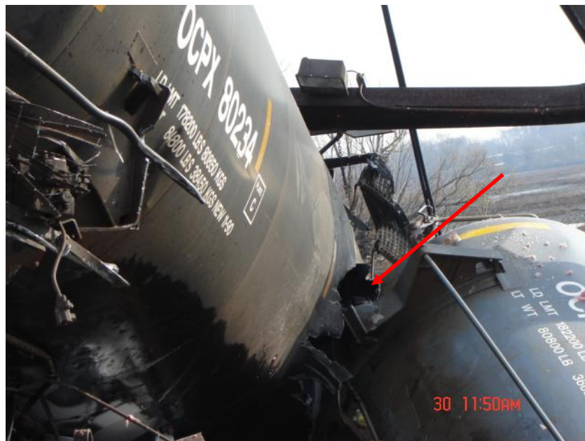
Figure 15 - Image of breach in OCPX 80234 on November 30, 2012. (Photograph courtesy of the FRA)
