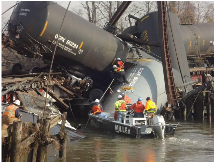
Figure 12 - Image of emergency responders climbing on tank car OCPX 80323 to inspect the breach in tank car OCPX 80234 at 10:49 a.m. on the morning of the accident. 46 (Photograph courtesy of the wife of the Paulsboro Assistant Fire Chief)
