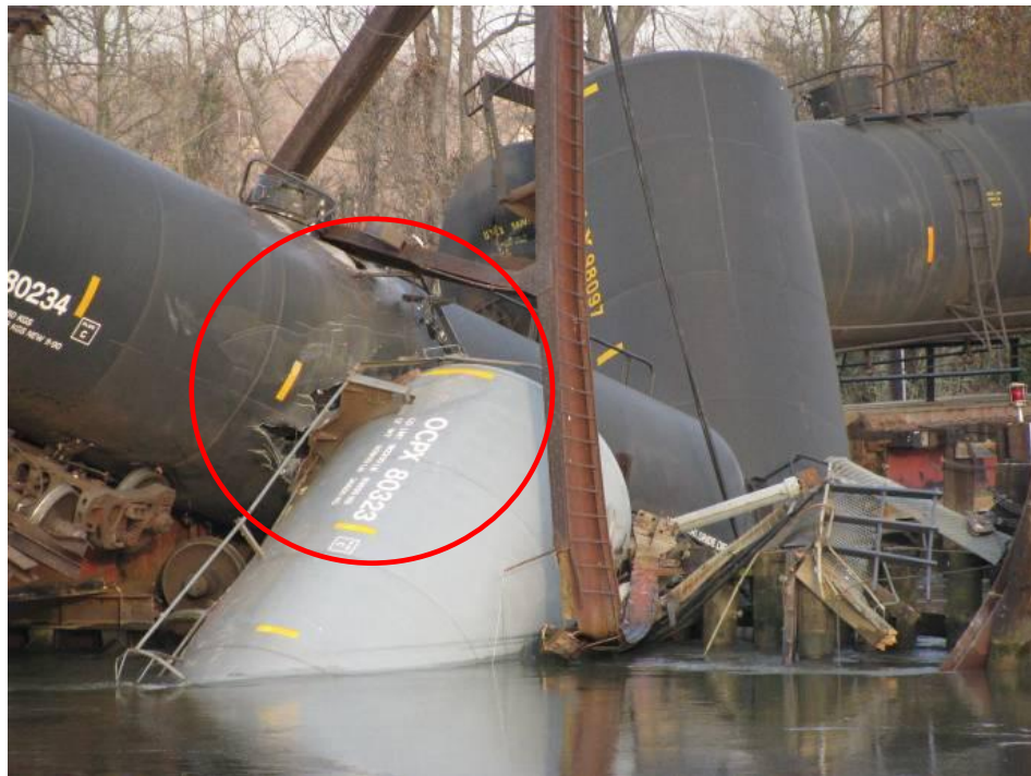
Figure 2 – Close-up photograph of tank car OCPX 80323 and the breach in tank car OCPX 80234 on November 30, 2012.
