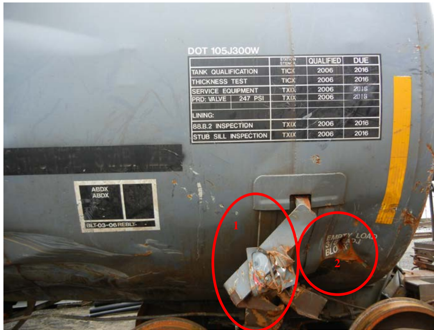
Figure 11: Close-up image of B-left body bolster and web deformation (labeled 1) and adjacent jacket puncture (labeled 2) in tank car OCPX 80323.
