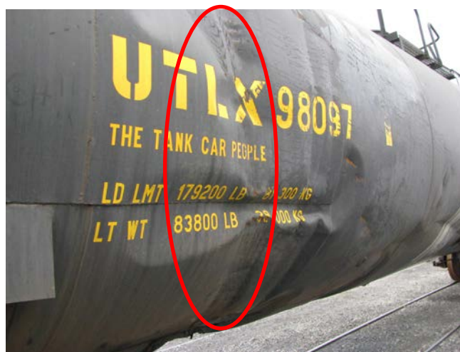
Figure 2: Example of discernable damage (highlighted in red) to tank car jackets as a result of crane lifting cables.
