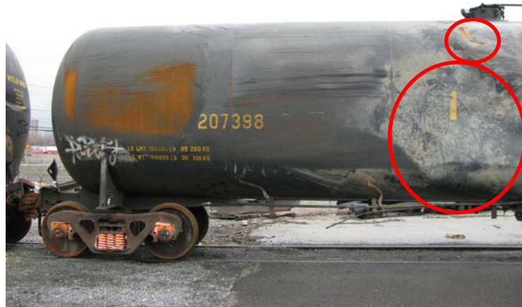
Figure 3: Scrapes above A-left body bolster and two oblong dents (highlighted in red) on tank car UTLX 207398.
