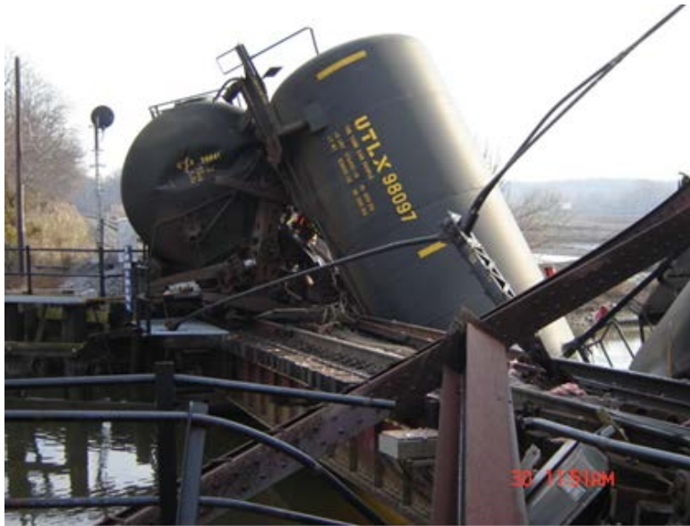
Figure 23: Final resting position of tank cars UTLX 98097 and UTLX 98041 after the accident.
