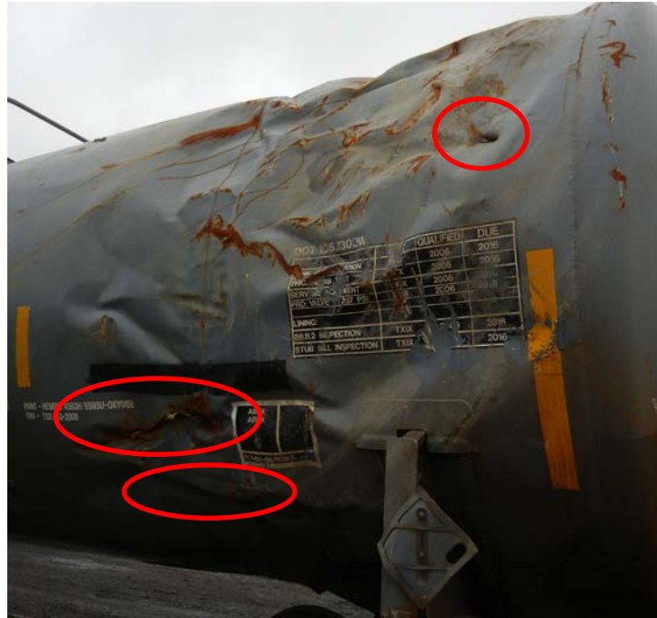
Figure 9: Gouges (highlighted in red) in tank jacket on A-right side of tank car OCPX 80323.
