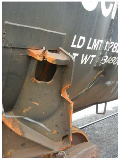
Figure 20: Inboard deformation of B-right body bolster on tank car OCPX 80234.
