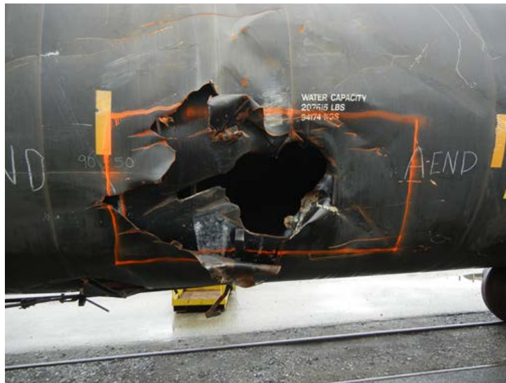
Figure 28: Portion of tank shell from OCPX 80234 (marked in orange) that was cut and sent to the NTSB Materials Laboratory in Washington, DC.
