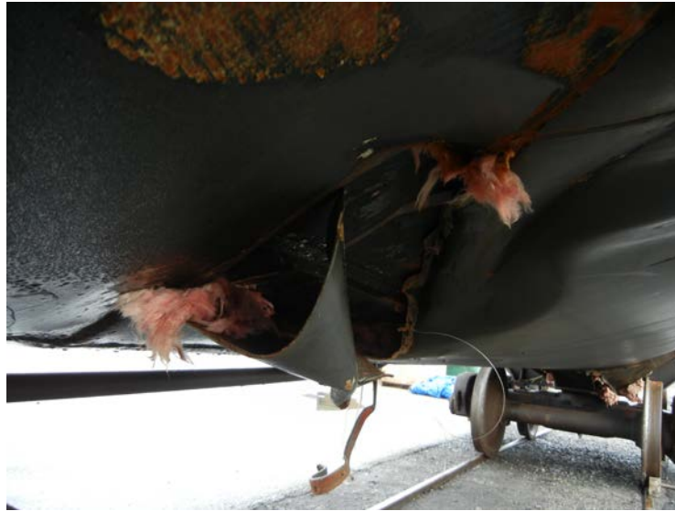
Figure 19: Triangular tear in the jacket at the bottom of the tank car OCPX 80234.
