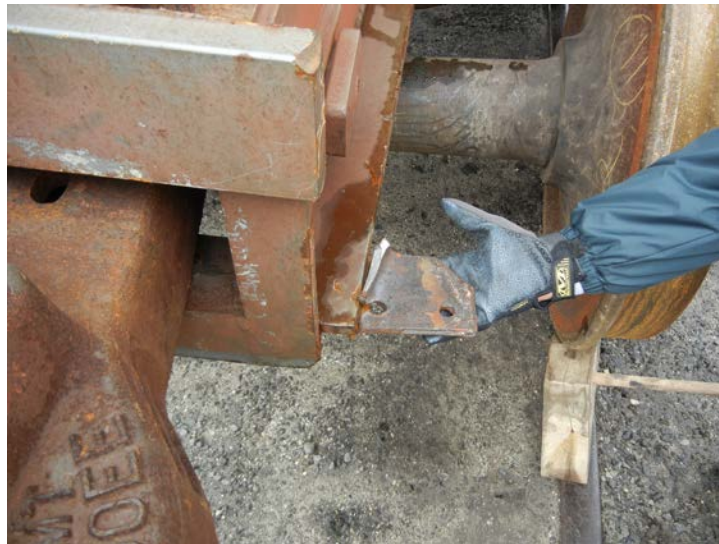
Figure 14: Recovered mounting plate that is ordinarily welded to tank car sill.
