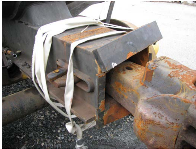
Figure 5: Damage to B-end striker plate on tank car UTLX 207398.
