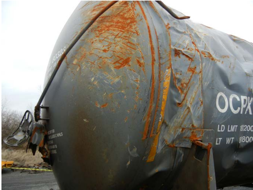
Figure 7: Damage to the B-end head shield and jacket on tank car OCPX 80323.
