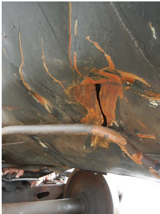
Figure 22: Line-shaped puncture of the jacket of OCPX 80234.
