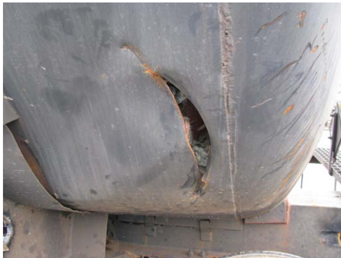
Figure 27: Tear near A-right head of tank car UTLX 98097.
