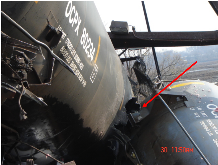
Figure 13: Breach in OCPX 80234 on November 30, 2012. (Photograph courtesy of the FRA)
