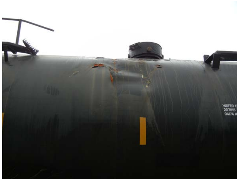
Figure 21: Damage to the top of tank car OCPX 80234 caused by the bridge A-frame.
