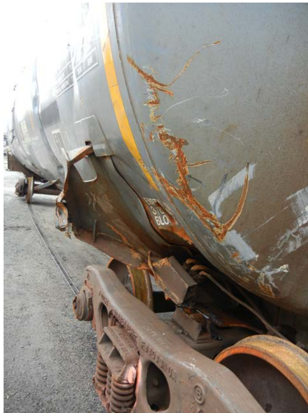
Figure 12: Scrapes on the B-head shield and damage to the B-Left side jacket of tank car OCPX 80323.
