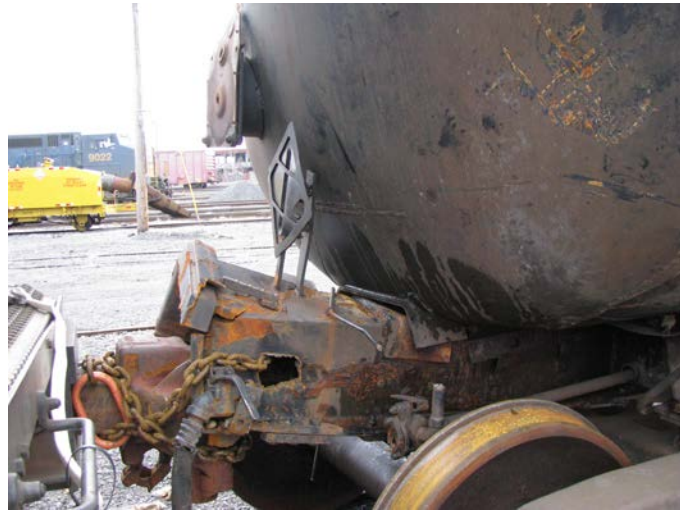
Figure 26: Damage to the B-end stub sill and striker plate of tank car UTLX 98097.
