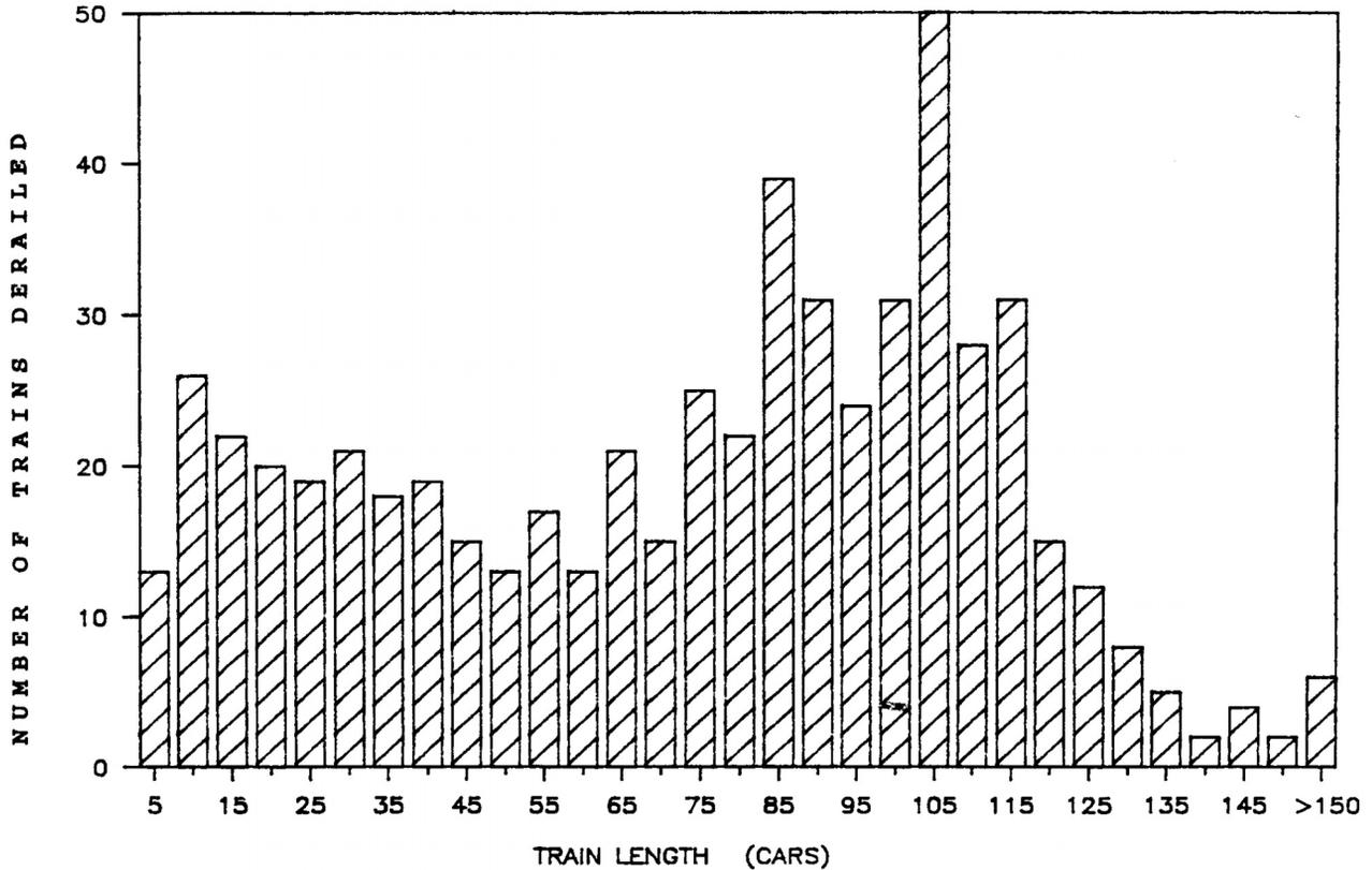
FIGURE 2 Train length distribution (CTC accident data 1980-1985).
