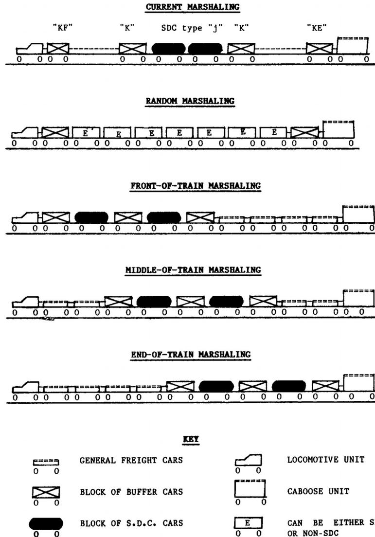
FIGURE 7 Alternative marshaling regulations considered.
