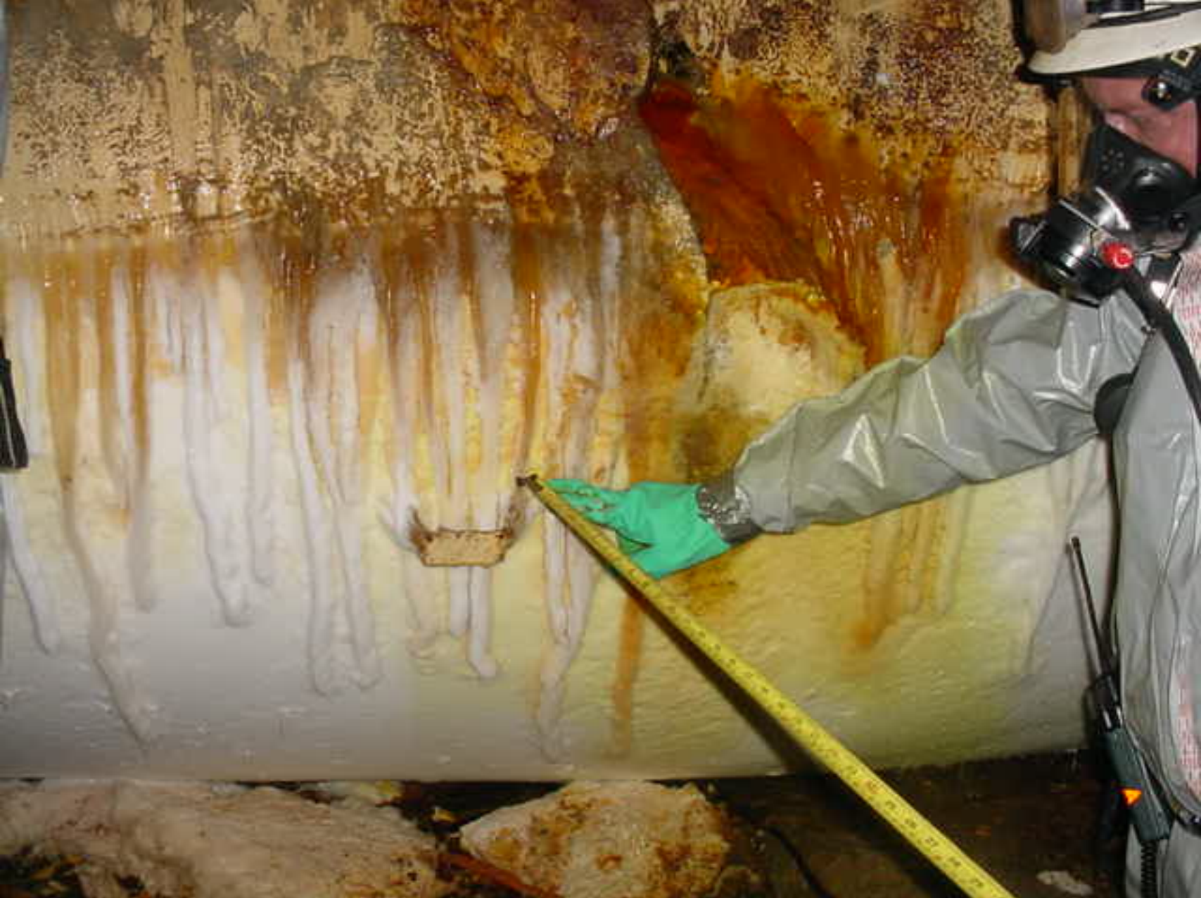
Haz/Mat Appx I - UTLX 900270 First Resp Liquid Chlorine Level Estimate
