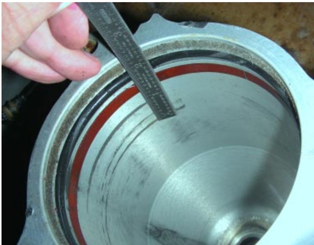
Photo 9. Right Cylinder Impact Marks on Piston
