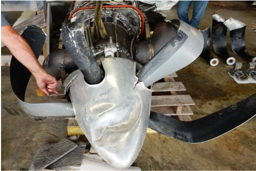
Photo #5 – Right propeller as-received
