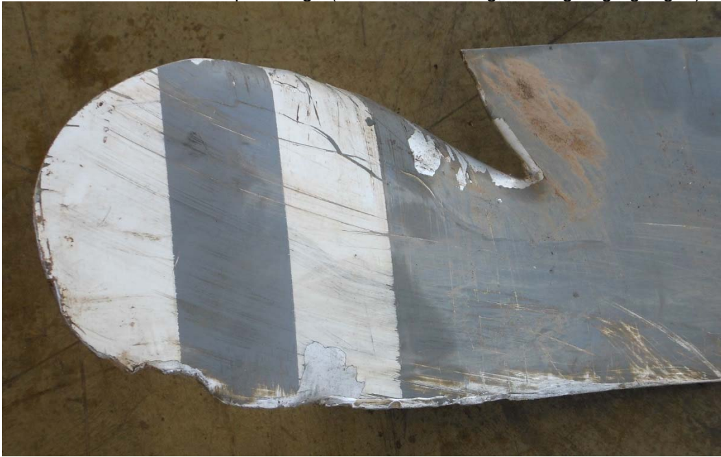
Photo #19 – R2 blade tip damage (chordwise scoring, leading edge gouges)
