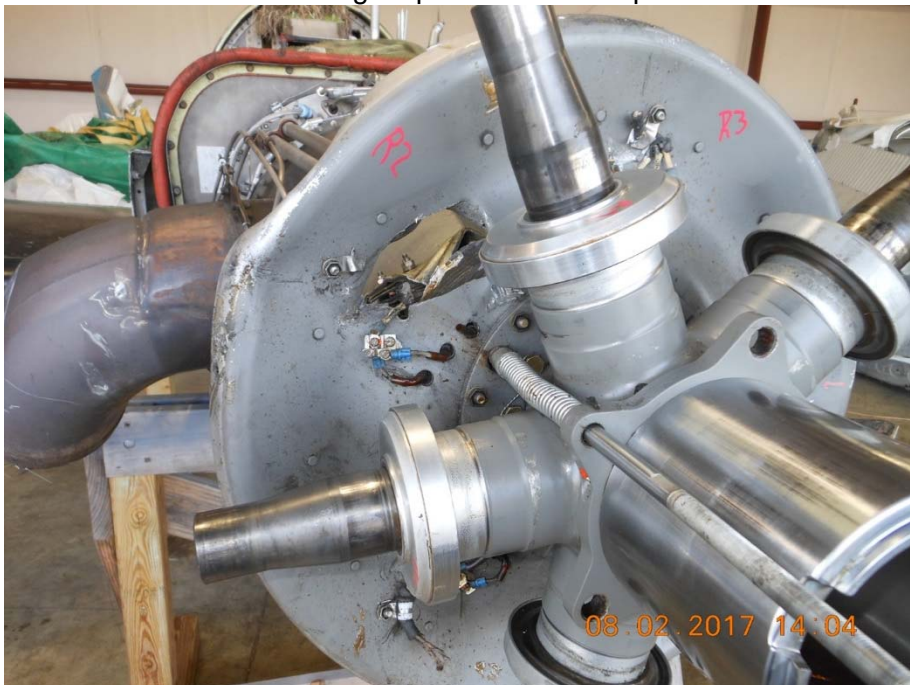
Photo #8 – Right spinner bulkhead puncture
