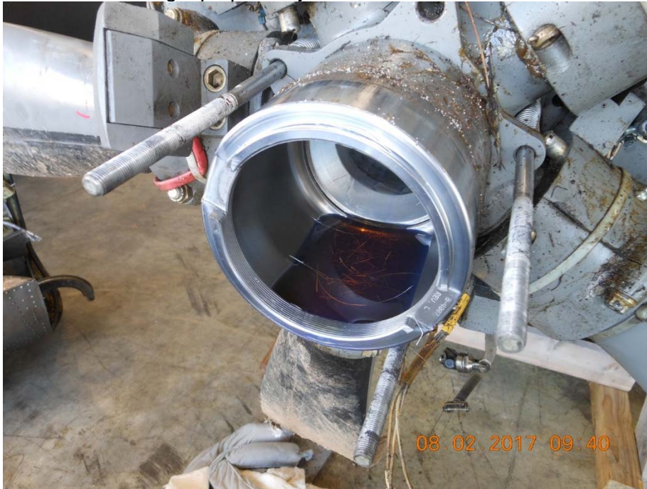
Photo #11 – Right propeller cylinder internal with thread whiskers
