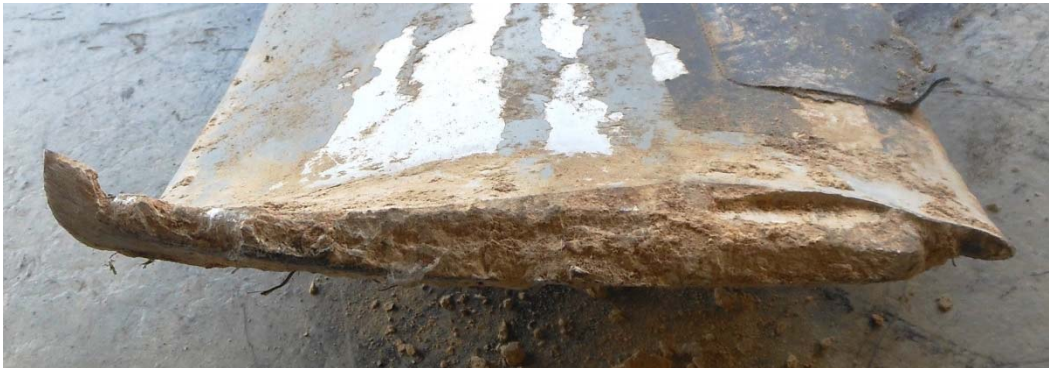
Photo #22 – R5 blade failure
