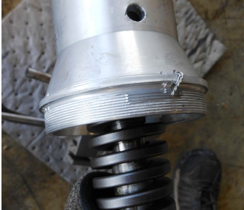
Photo #13 – Right propeller forward spring cup stripped threads
