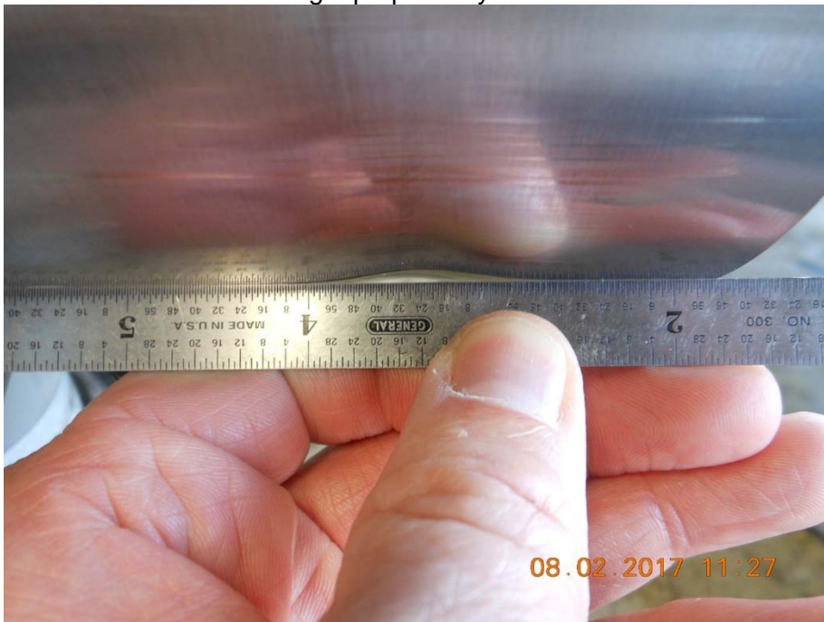
Photo #12 – Right propeller cylinder crease/dent
