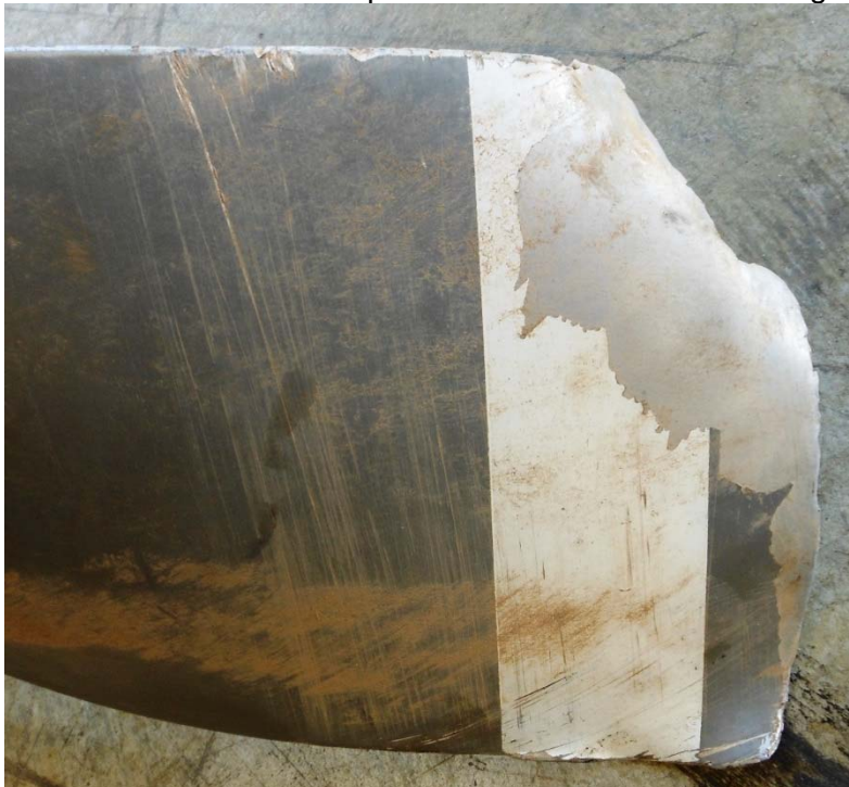
Photo #18 – R1 blade tip fracture and chordwise scoring
