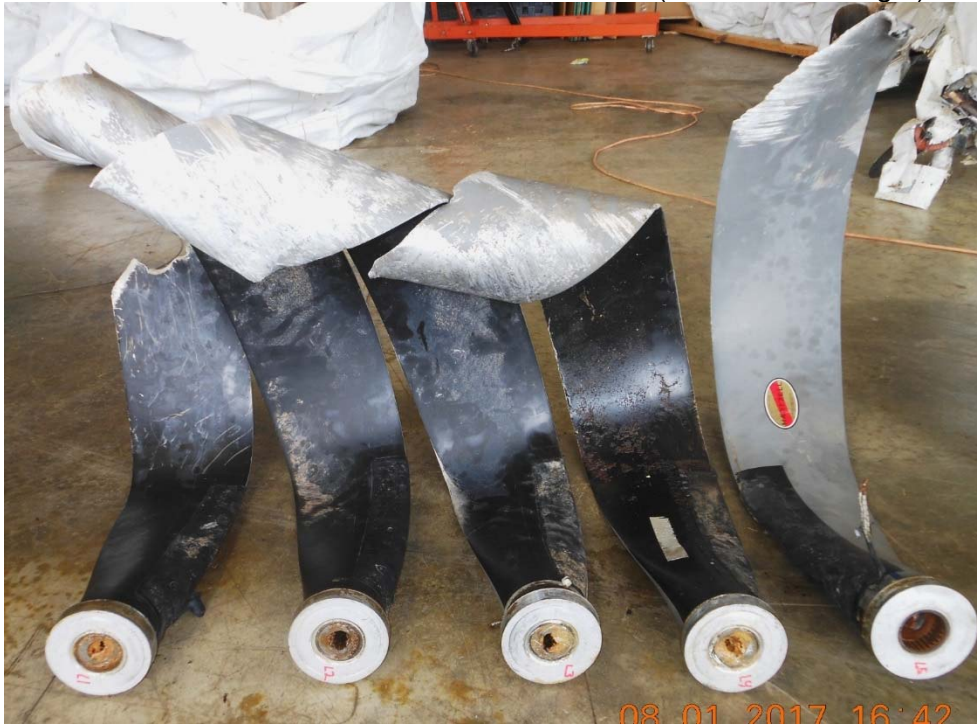
Photo #38 – Left blades view of tip areas (L5 to L1 left to right)
