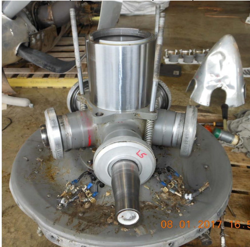
Photo #35 – Left propeller hub assembly with one pilot tube intact
