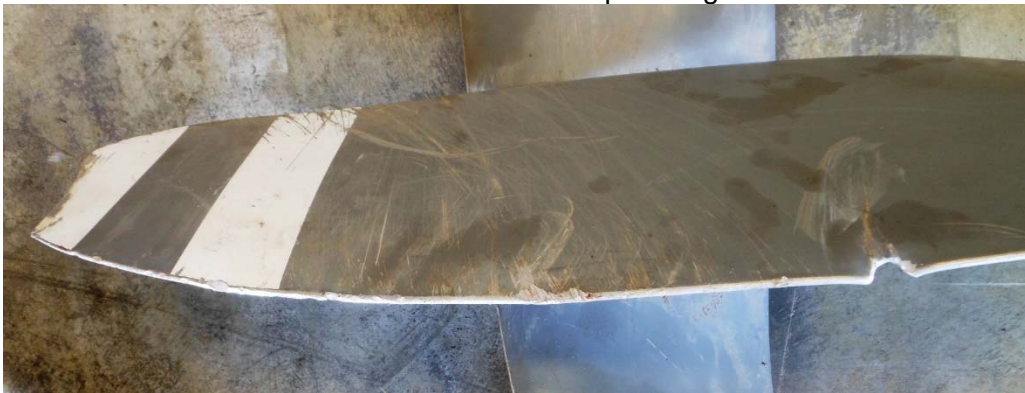
Photo #20 – R3 blade tip damage
