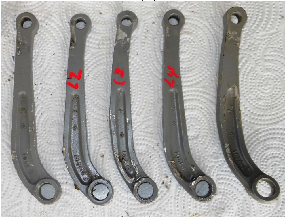
Photo #31 – Left propeller link arms
