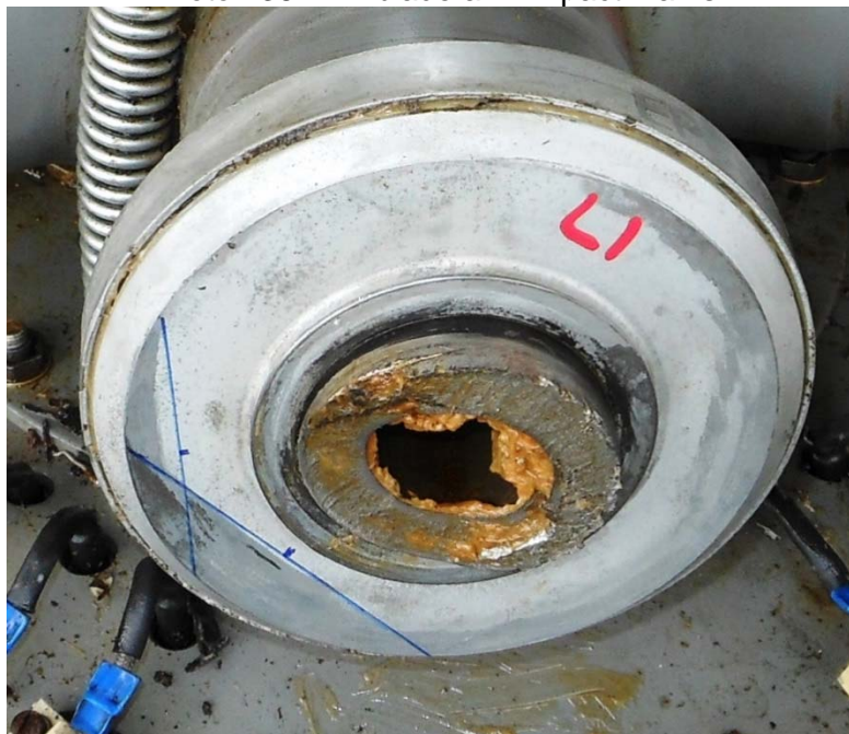
Photo #36 – L1 blade arm impact marks
