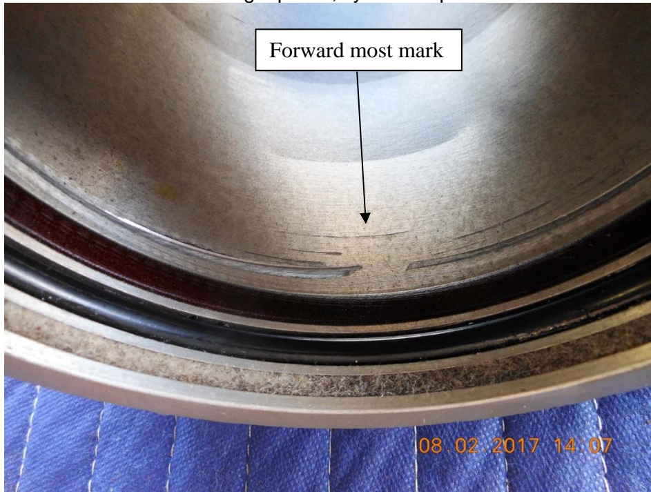
Photo #9 – Right piston, cylinder impact marks
