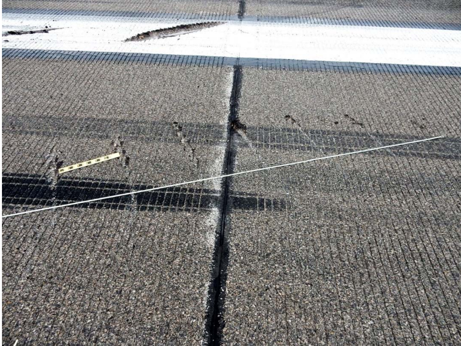
Photo #1 – Left Propeller Strike Marks in Runway (photo courtesy of NTSB)
