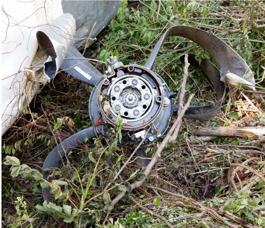
Photo #2 – Left propeller and forward RGB in-situ (photo courtesy of NTSB)
