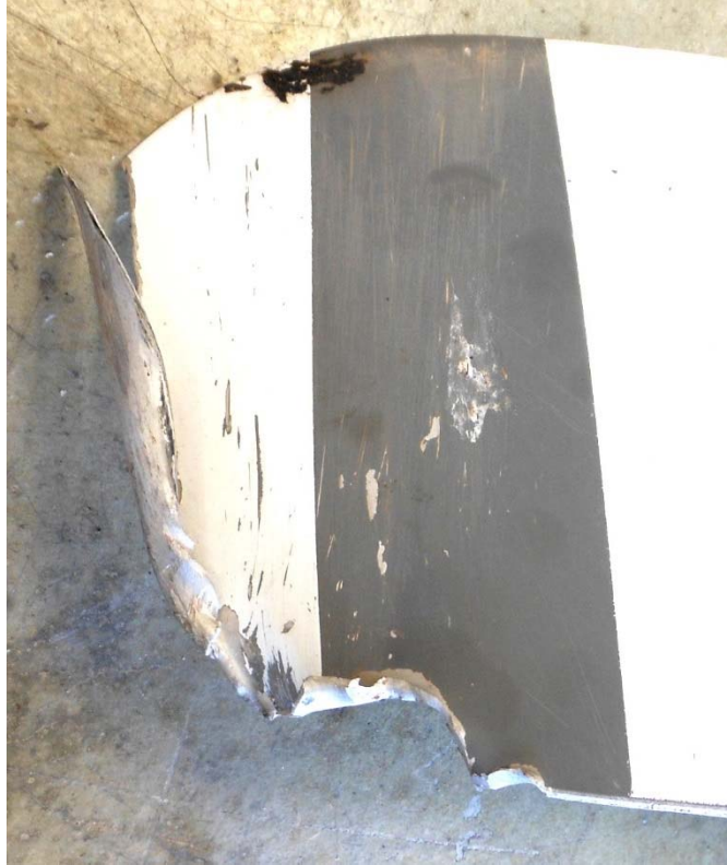
Photo #21 – R4 blade tip damage
