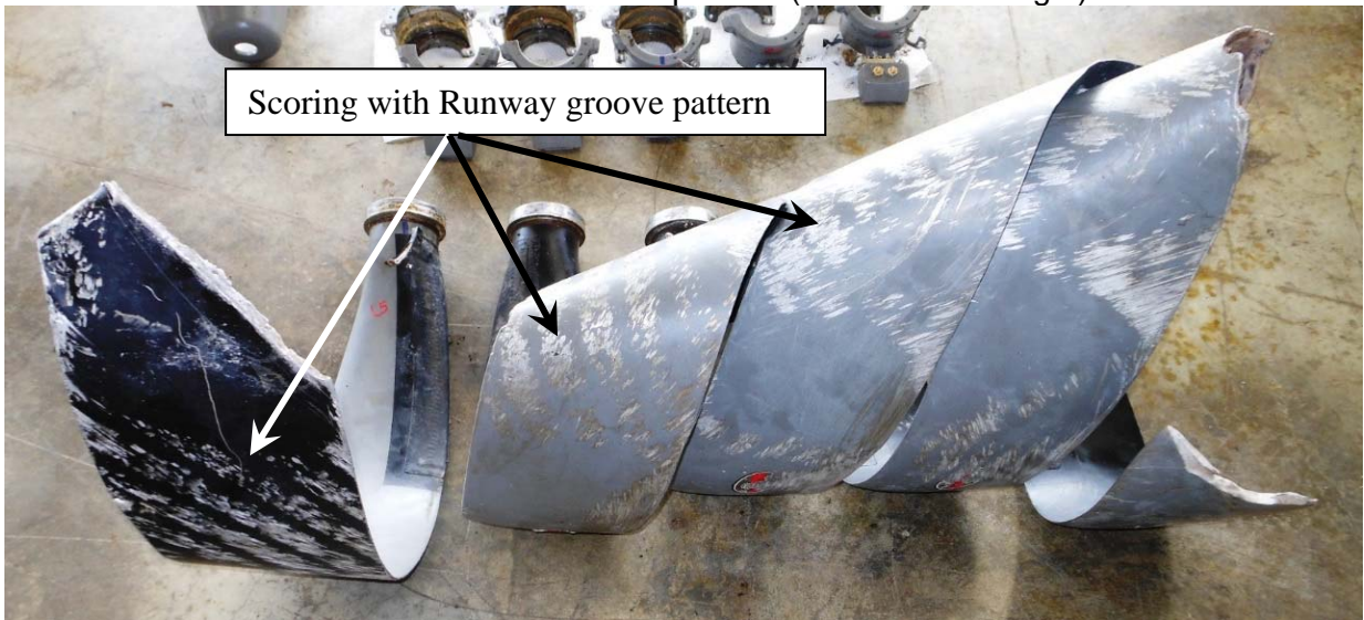
Photo #38 – Left blades view of tip areas (L5 to L1 left to right)
