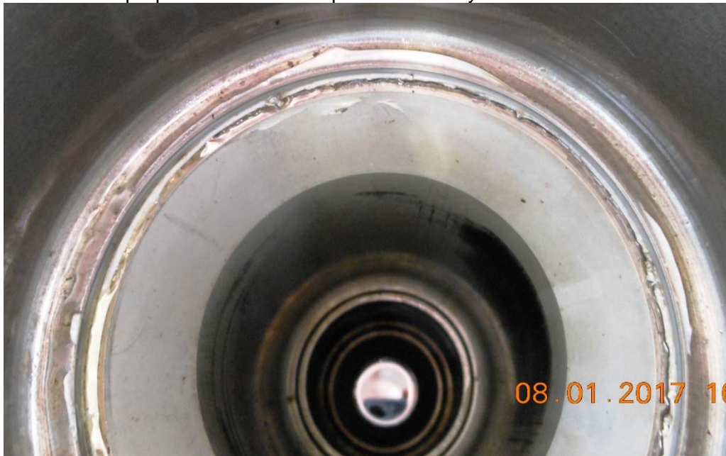
Photo #30 – Left propeller white RTV squeeze-out at cylinder/hub threaded connection
