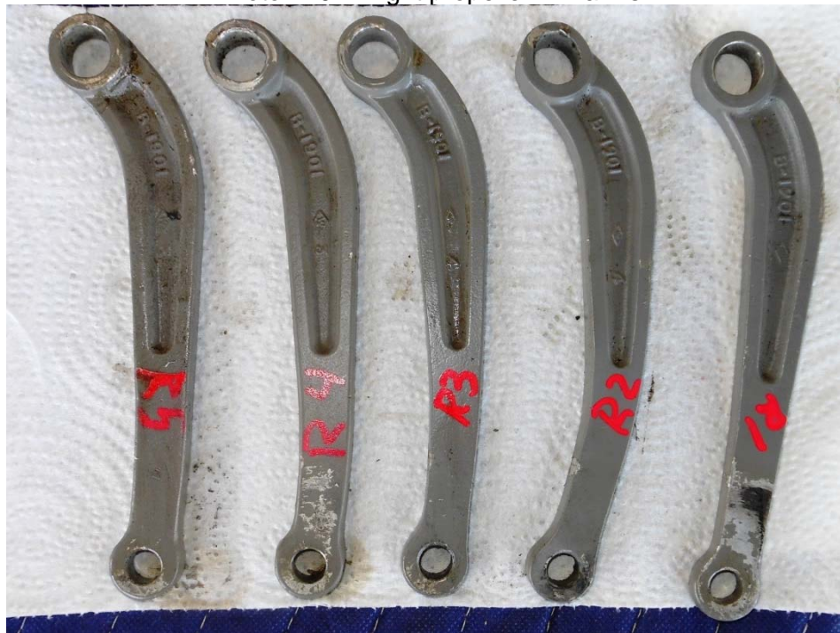
Photo #10 – Right propeller link arms
