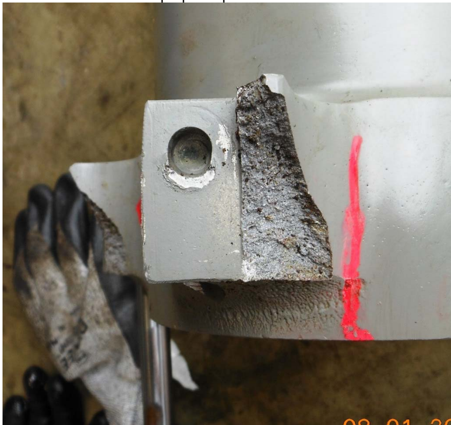
Photo #28 – Left propeller piston link arm fracture at L1
