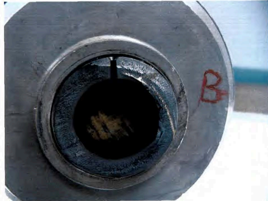
View of Pilot tube fractures, as received, and prior to removal for examination. Both tubes fractured immediately adjacent to the Hub face.
