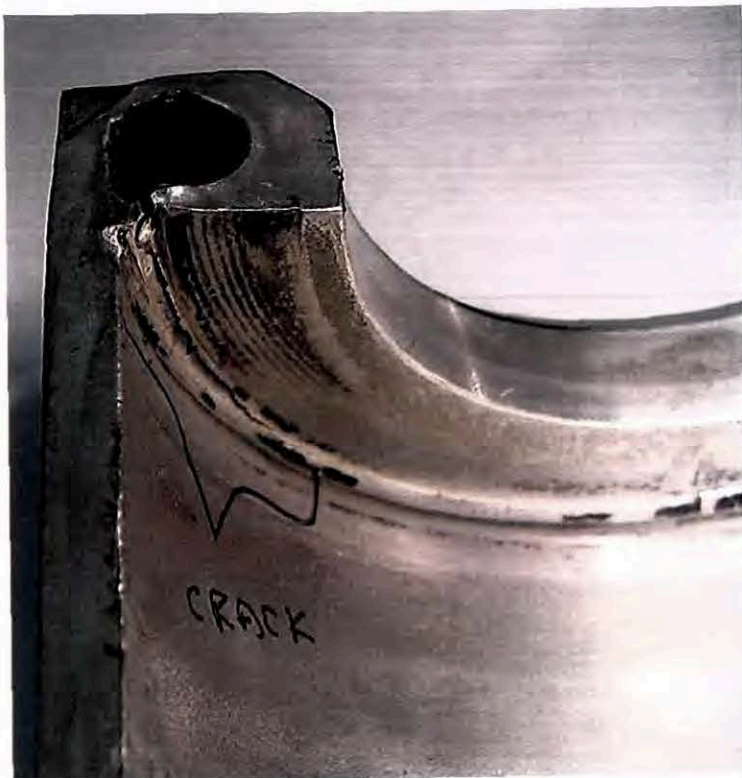
The crack extends from the bolt hole region and is accompanied by a considerable amount of plastic deformation.
