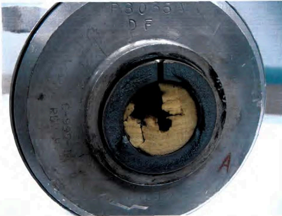
View of Pilot tube fractures, as received, and prior to removal for examination. Both tubes fractured immediately adjacent to the Hub face.
