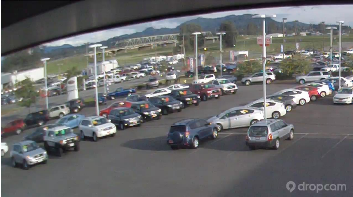
Image 4.13: Vertical lines from light pole positions 1 and 2 are used to indicate when the Accident Combination Unit crossed each segment from point INT1 to INT2 on the centerline of the outermost lane of Interstate 5 southbound. Here, the Accident Combination Unit is seen at point INT1, a checkpoint using Light Pole #1 as a reference position. The indicated video time is 34 seconds and 11 frames.
