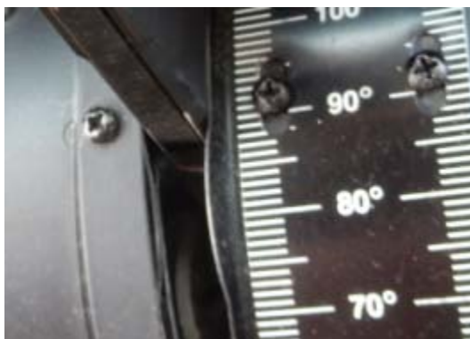
FIGURE 1 – G10 THROTTLE PROTRACTOR POSITION (GL UNLATCHED/THROTTLE INTERLOCK)
