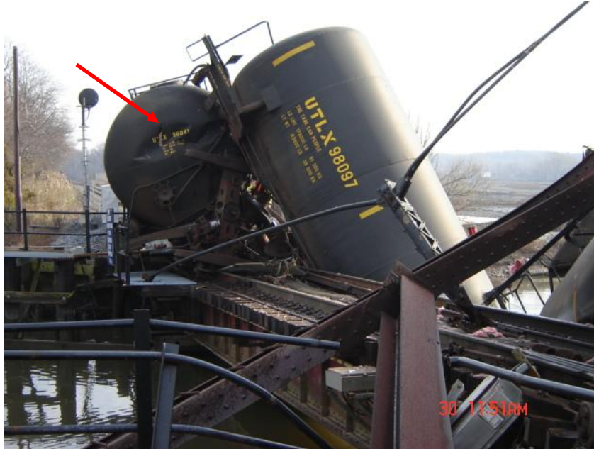
Figure 16 - Image of head damage to UTLX 98041 on November 30, 2012. (Photograph courtesy of the FRA)
