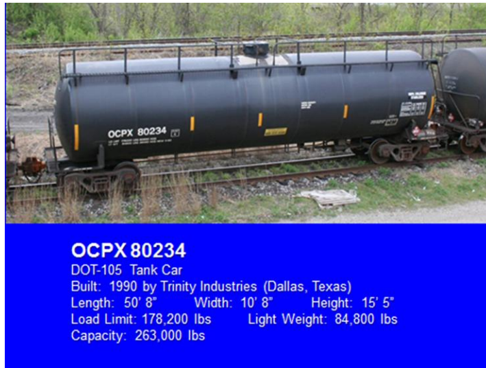
Figure 14 – Image of OCPX 80234 prior to the November 30, 2012, accident. (Photograph courtesy of the USCG)
