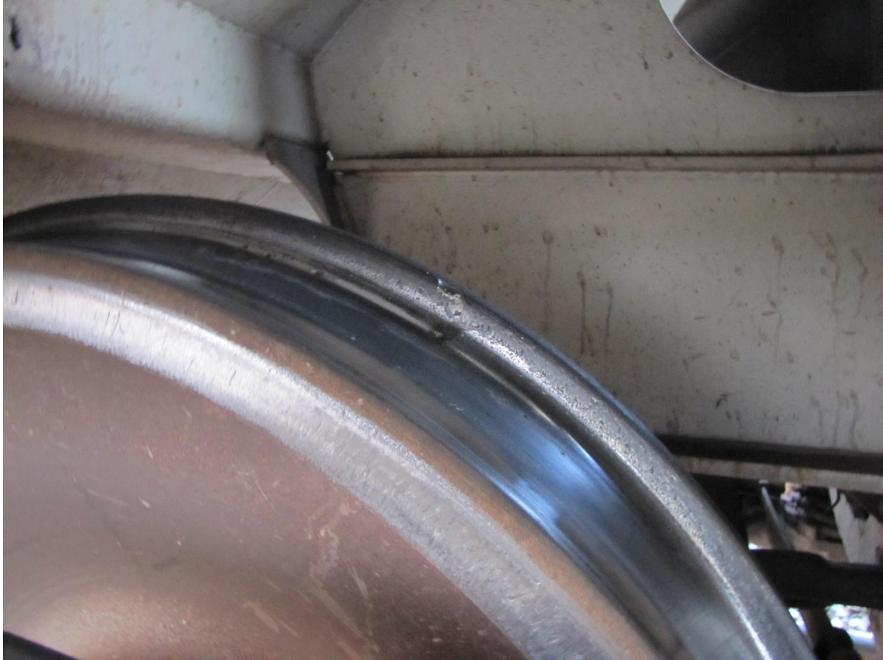
Figure 6-Typical impact marks on the flanges of three wheels of the fourth and fifth rail cars
