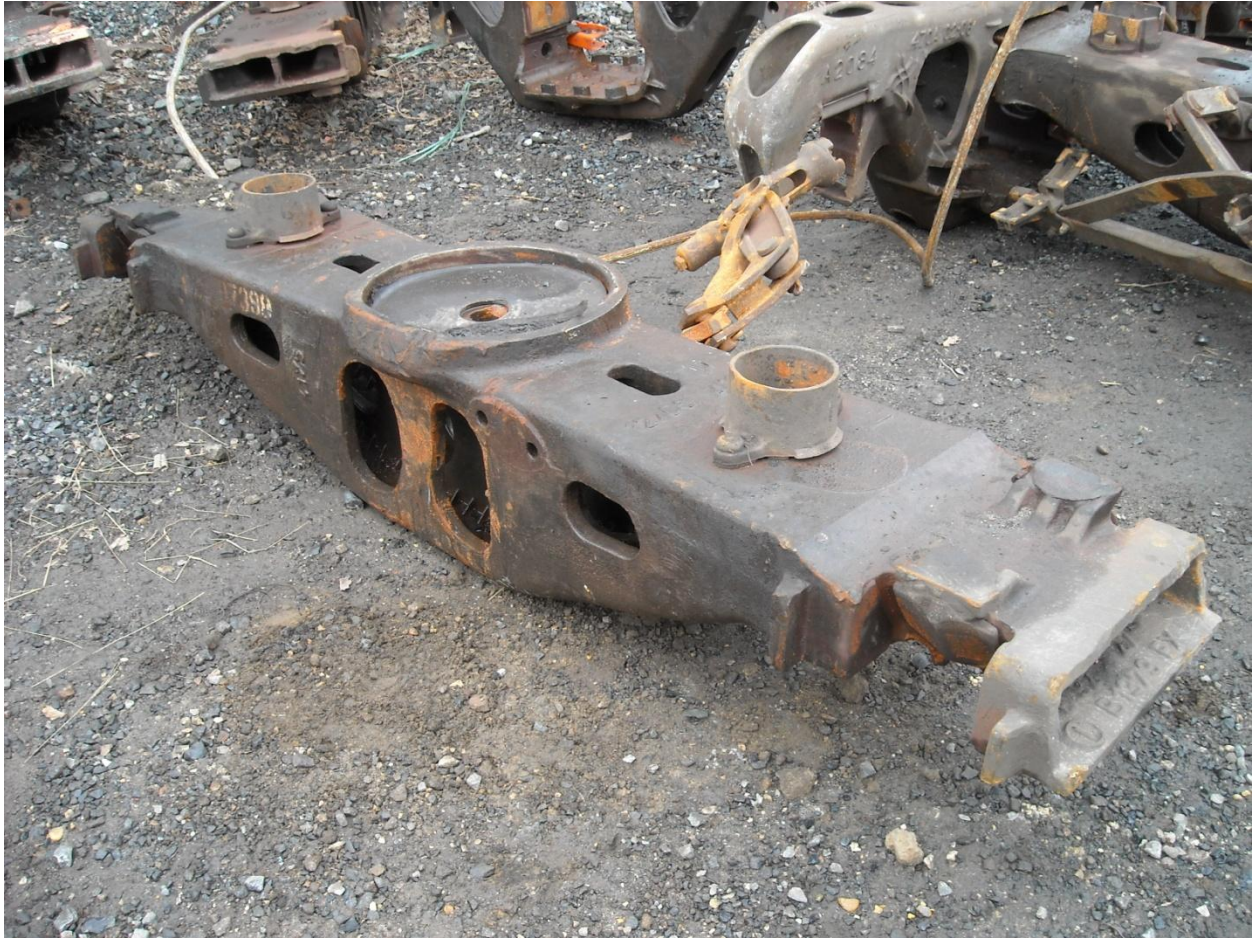
Figure 10 Typical recovered body bolster.
