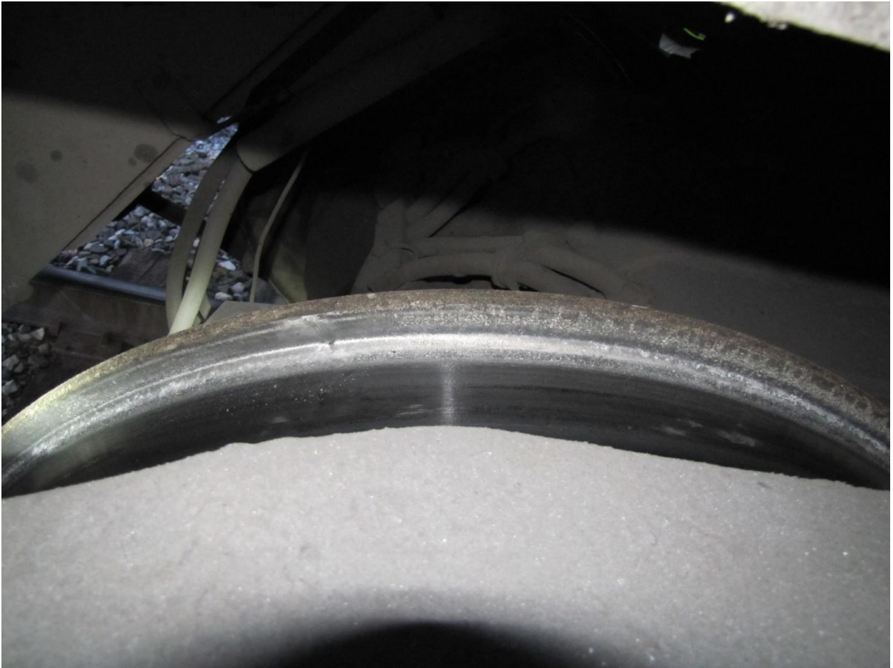
Figure 5-Typical impact marks on the flanges of three wheels of the fourth and fifth rail cars
