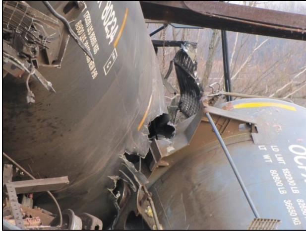
Figure 4-OCPX 80234 Torn open by OCPX 80323
