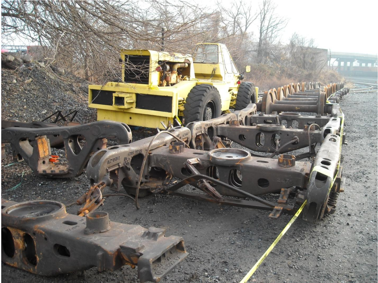
Figure 9 Recovered bolster, side frame, partial trucks and wheel sets.
