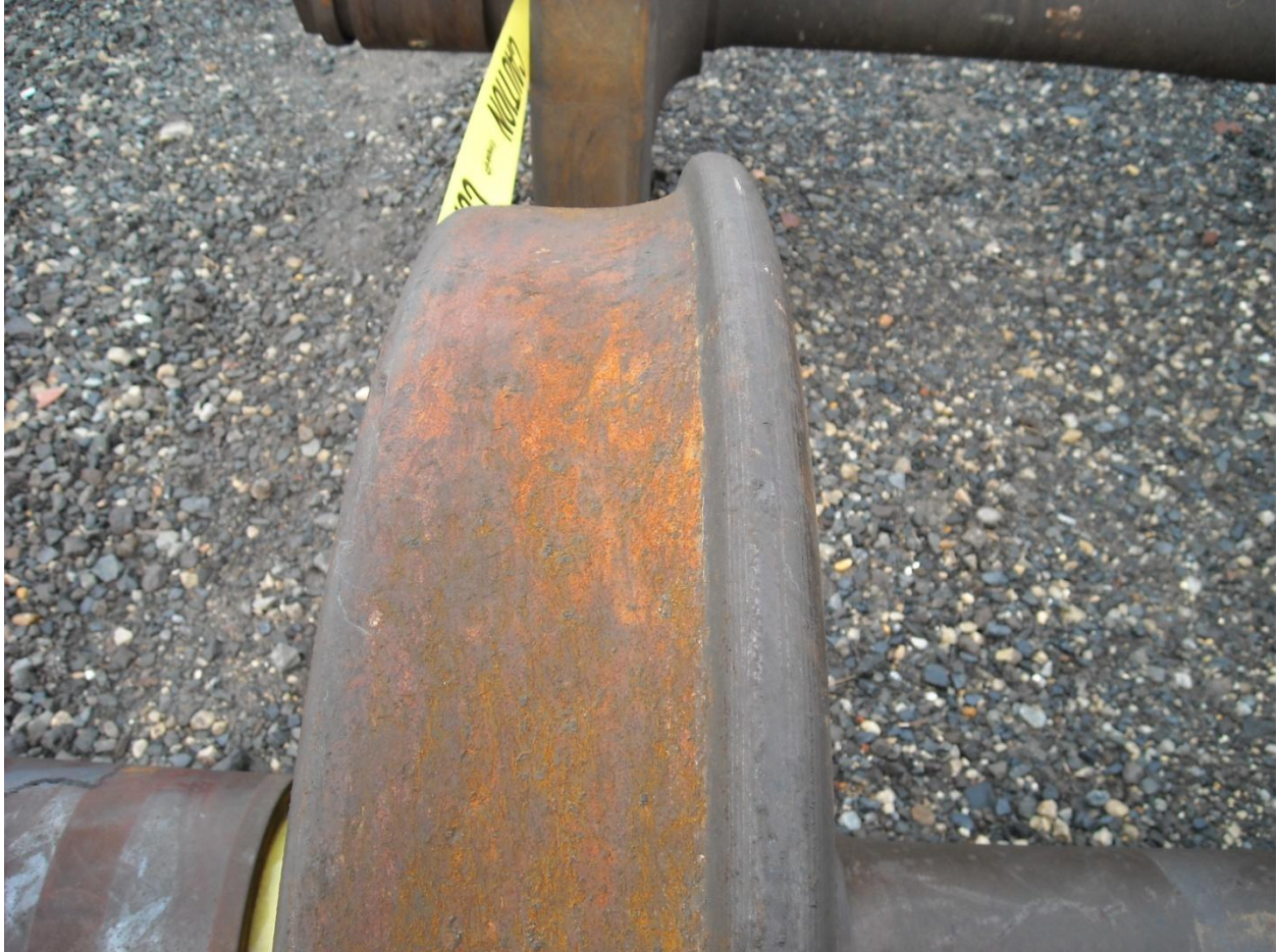
Figure 8 Typical recovered wheel profile.
