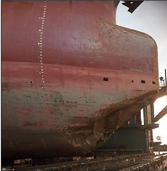
Damage to Nenita's bulbous bow starboard side. (Photo by Spring Marine Bulk, S.A.)
