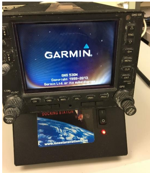
Figure 3. The Garmin GNS-530W after being repaired.
