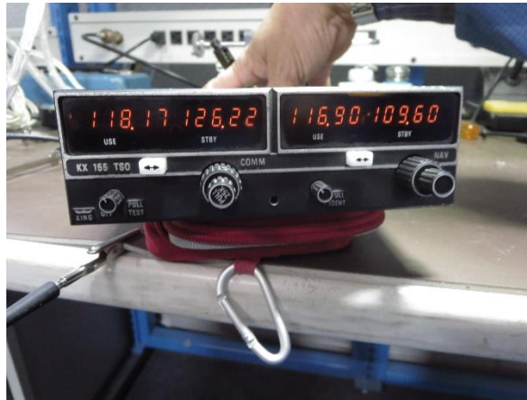
Figure 2. The device displaying the retained communications and navigational frequencies.
