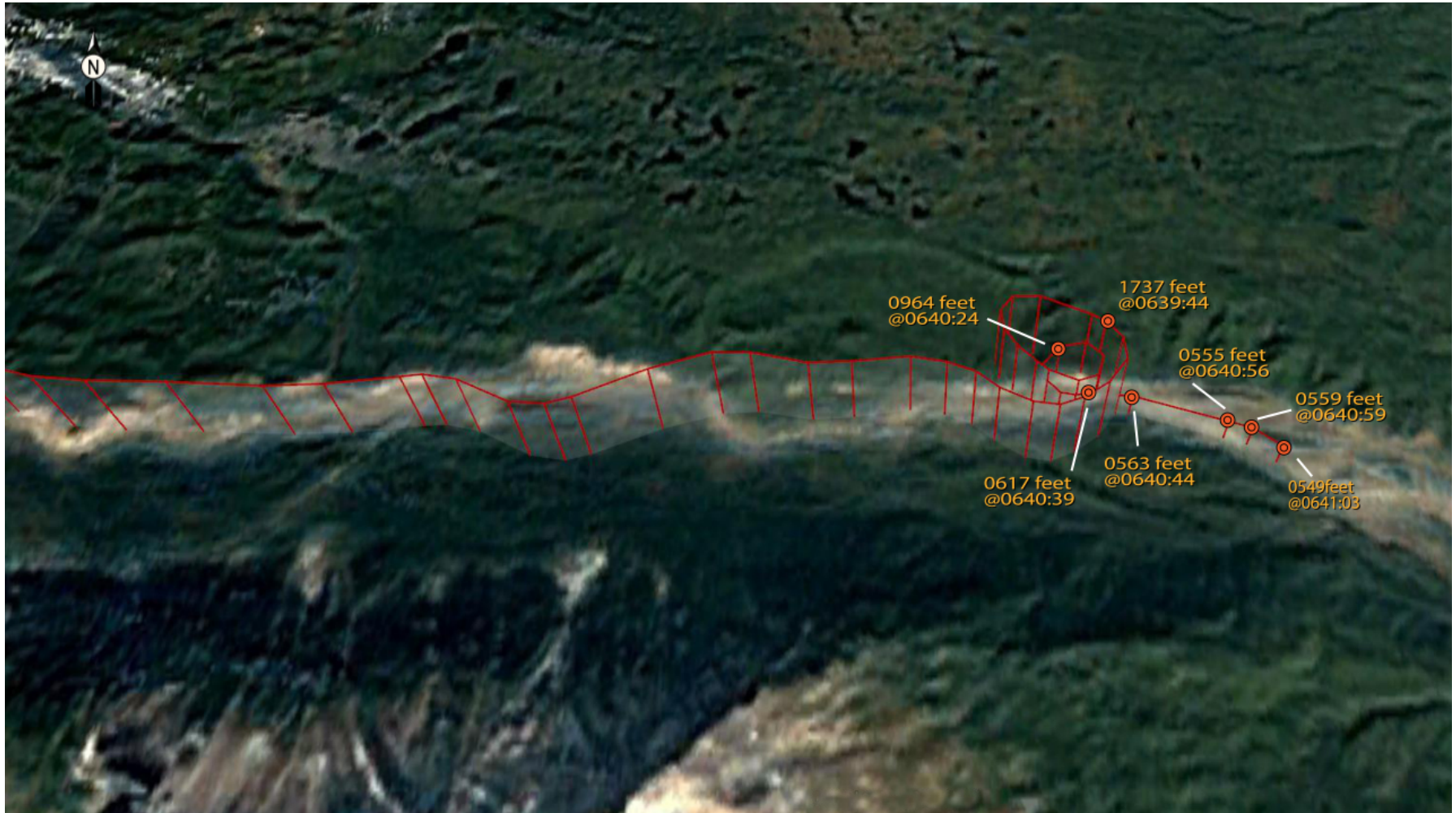
Figure 7. Google Earth overlay of the last segment of the accident flight with altitude and time of selected points in large scale
