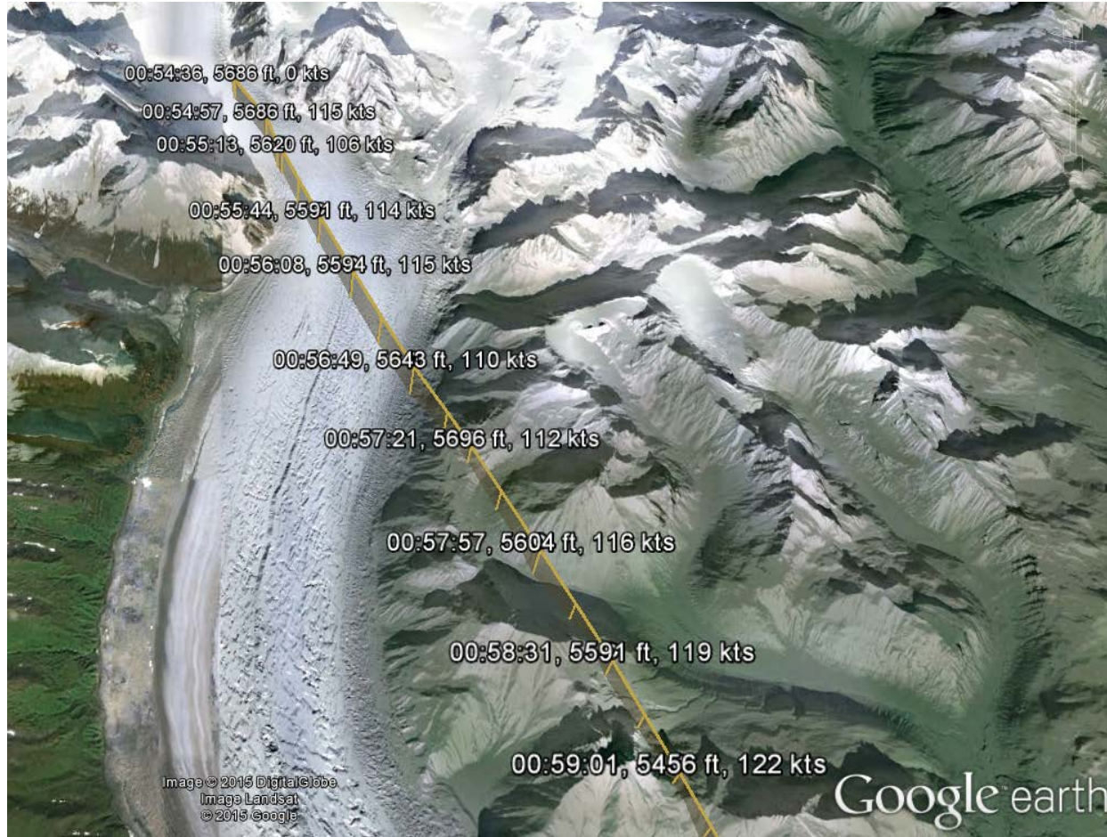
Figure 4. Google Earth overlay showing the beginning of the accident flight.
