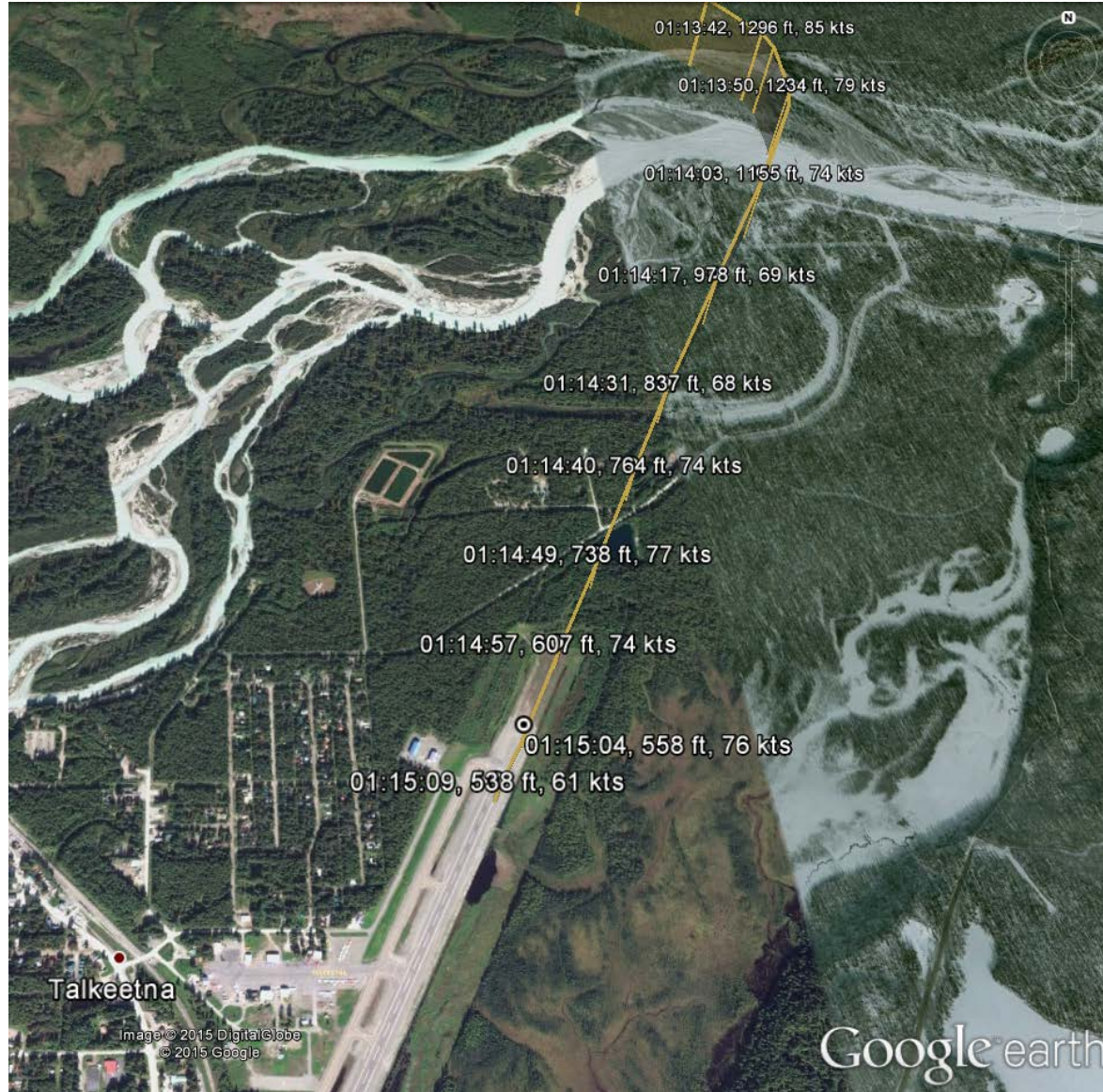
Figure 5. Google Earth overlay showing the end of the accident flight.
