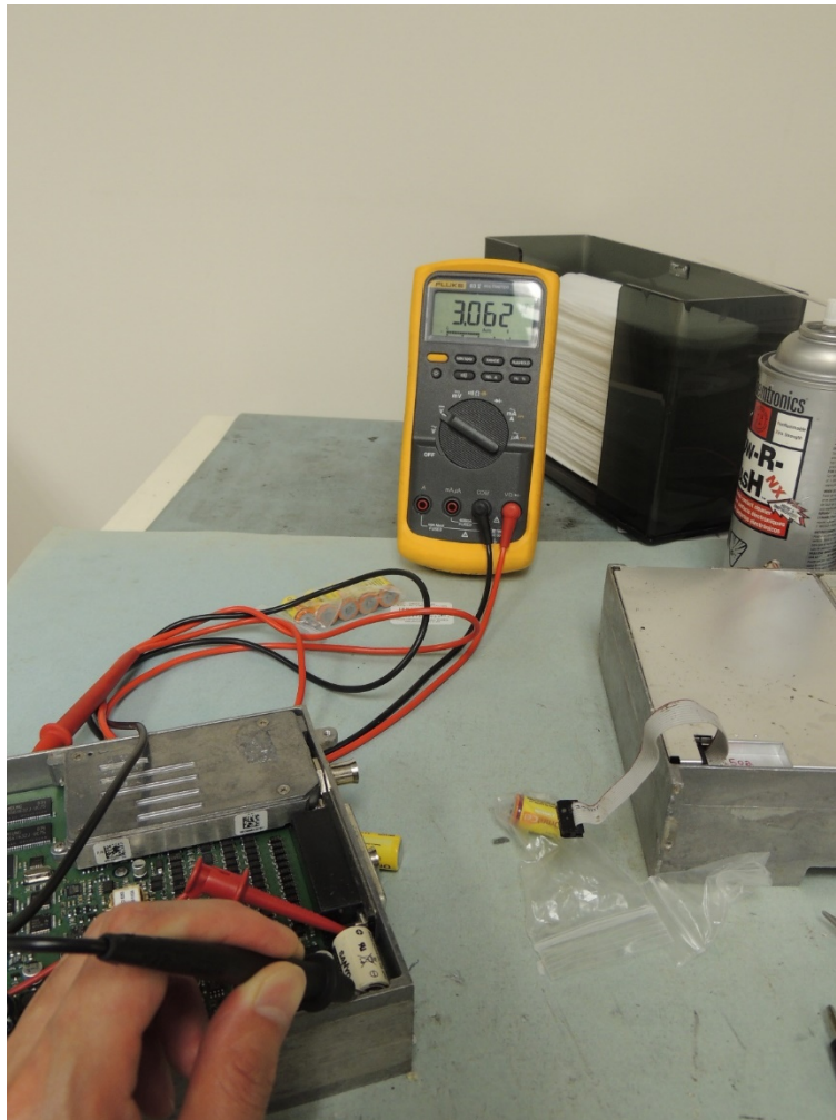
Figure 3. Internal backup battery attached and provided power
