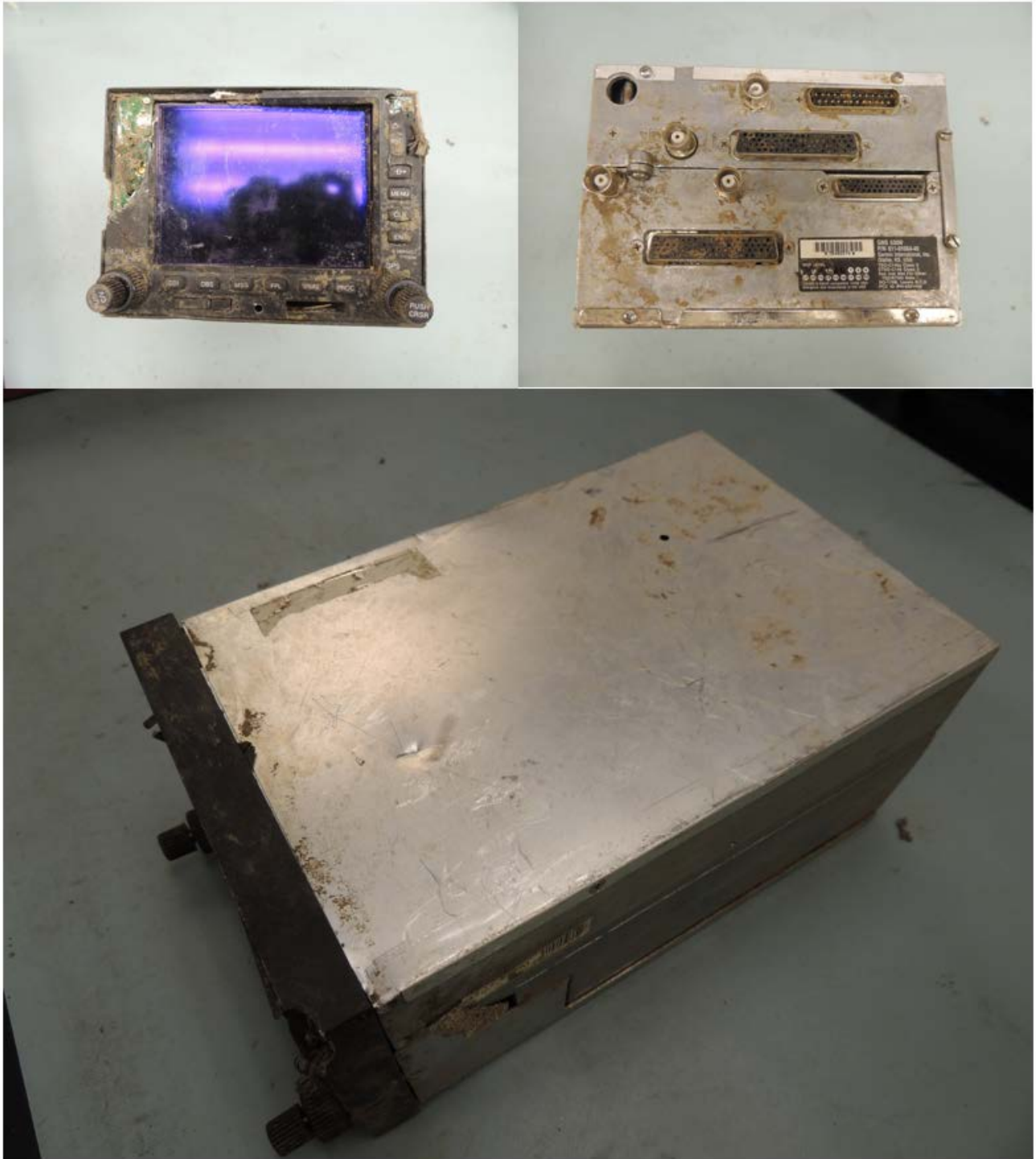
Figure 1. Front, back and body of Garmin GNS 530 as received
