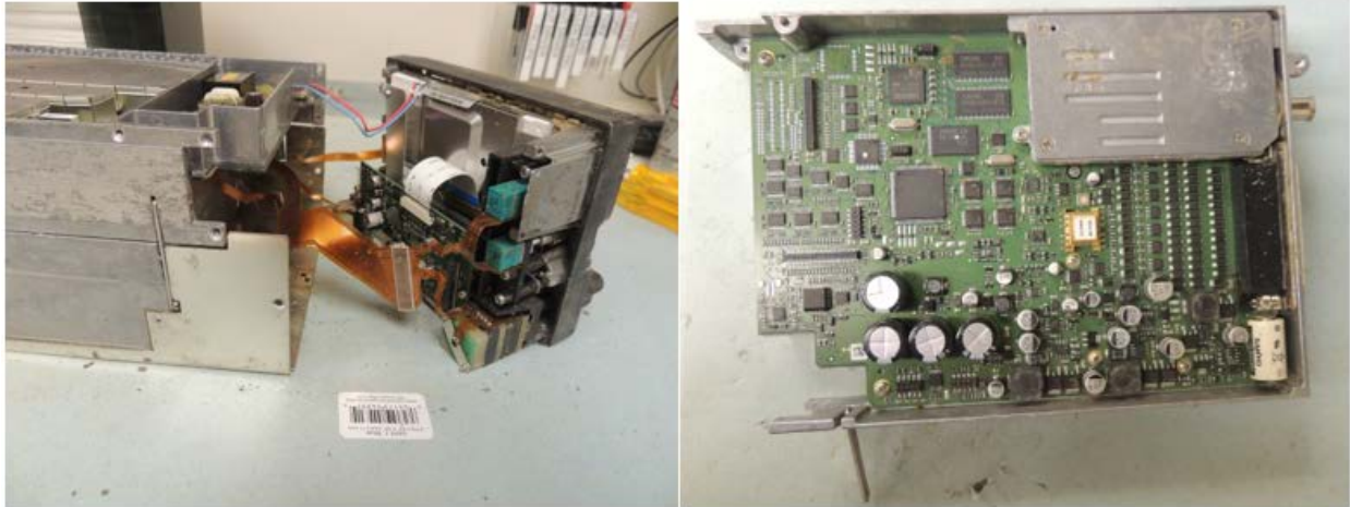
Figure 2. Interior of Garmin GNS 530 as received
