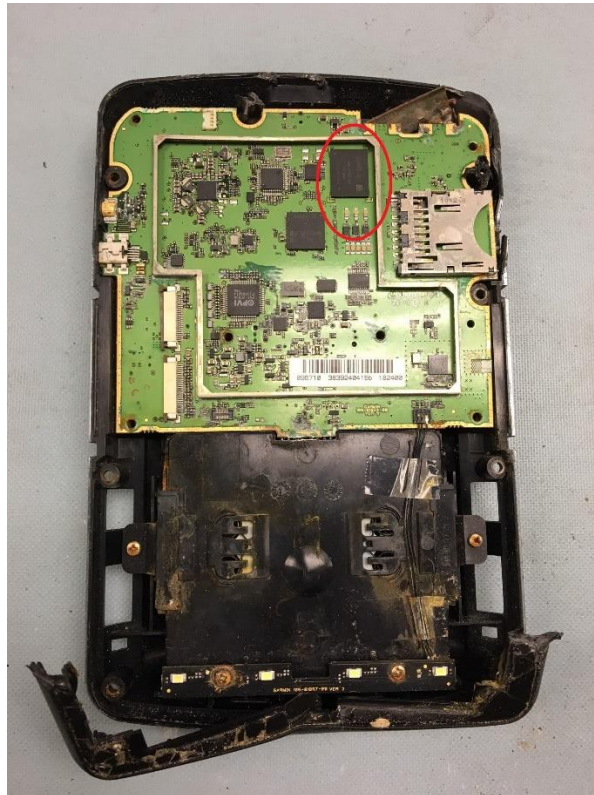
Figure 2. Photo of Garmin aera 796 main memory board with memory chip circled in red.
