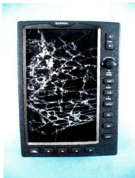
Figure 1. Photo of damaged Garmin GPSMAP 696.
