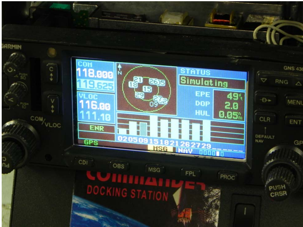
Figure 2: Garmin GNS 430 with power applied showing last COM and VLOC settings
