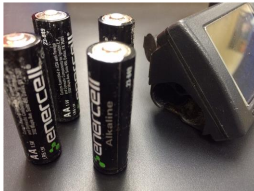
Figure 2. Photo of the device's battery housing area with corrosion present on the "AA" style batteries.
