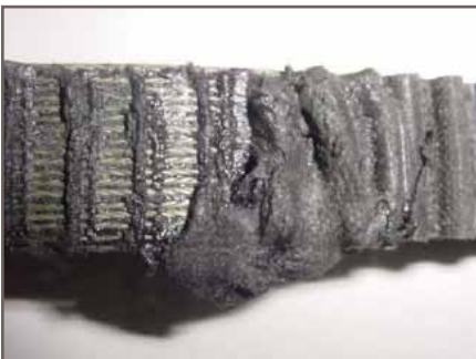
Figure 18 - Melting from high temperature operation, polyurethane
