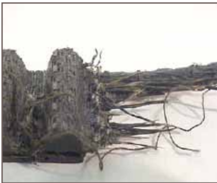
Figure 4 – Typical shock load failure
