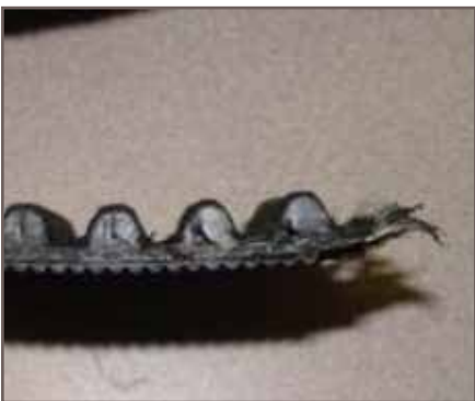
Figure 5 – Tooth root crack propagation
