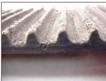
Figure 9 – Excessive tooth wear
