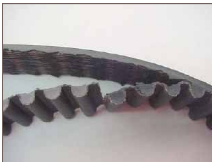
Figure 8 – Tooth separation failure
