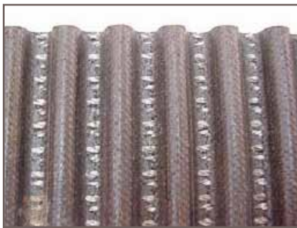
Figure 7 - Excessive land area wear
