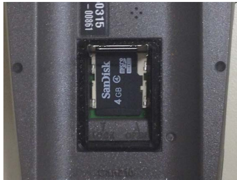
Figure 2. Garmin Rhino 530HCX GPS and Radio – microSD Card.
