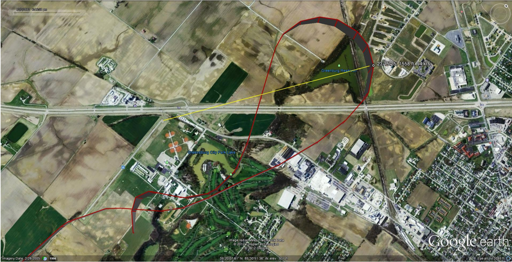
Figure 9. Google Earth overlay showing maximum distance of flight path north of airport from I34 runway threshold.
