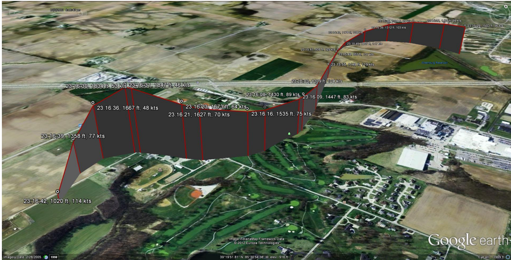
Figure 8. Google Earth overlay of second segment of aircraft path north of the airport until end of recording.
