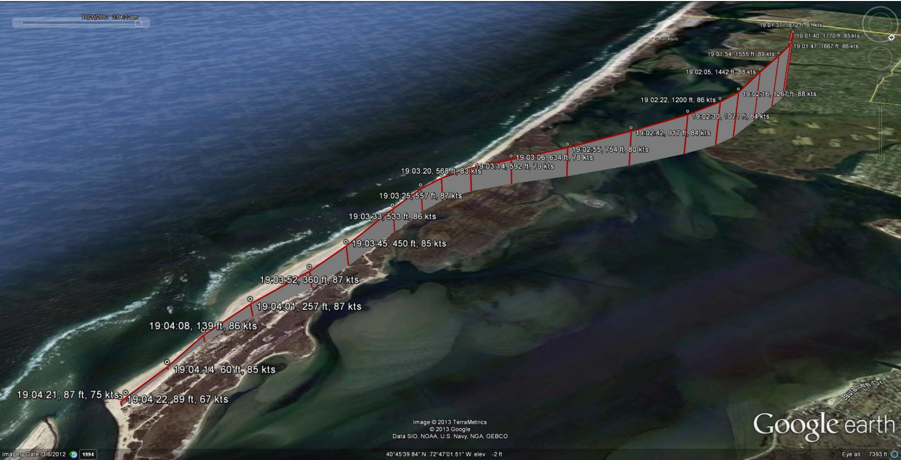
Figure 4. Google Earth overlay of the end of the accident flight recording.
