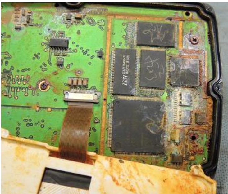
Figure 1. Photo of corrosion damage.
