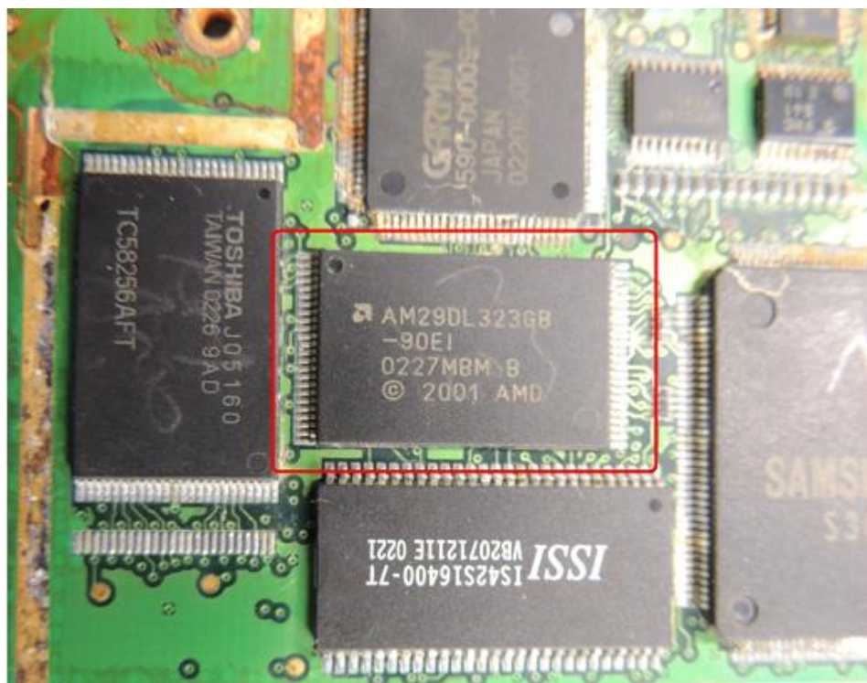
Figure 2. Photo of main non-volatile memory chip after cleaning.
