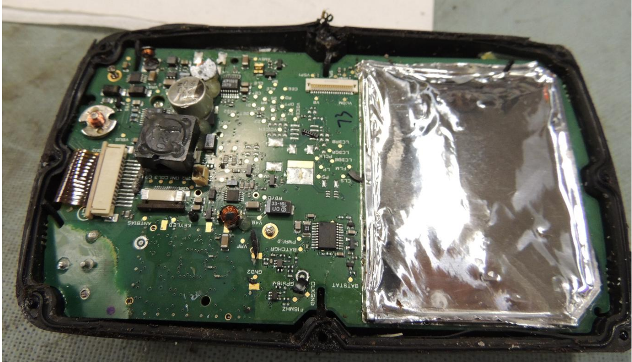
Figure 3. Photo of internal damage to PCB.
