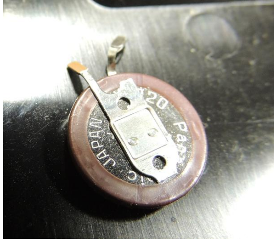
Figure 2. Internal inspection - button battery disconnected.
