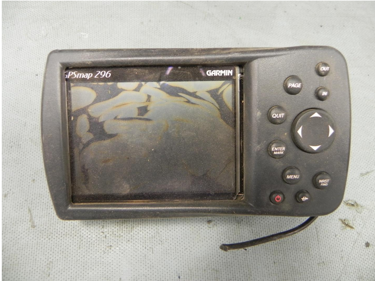
Figure 1. External view of the Garmin GPSMAP 296 (67008540) showing damage to the LCD display.
