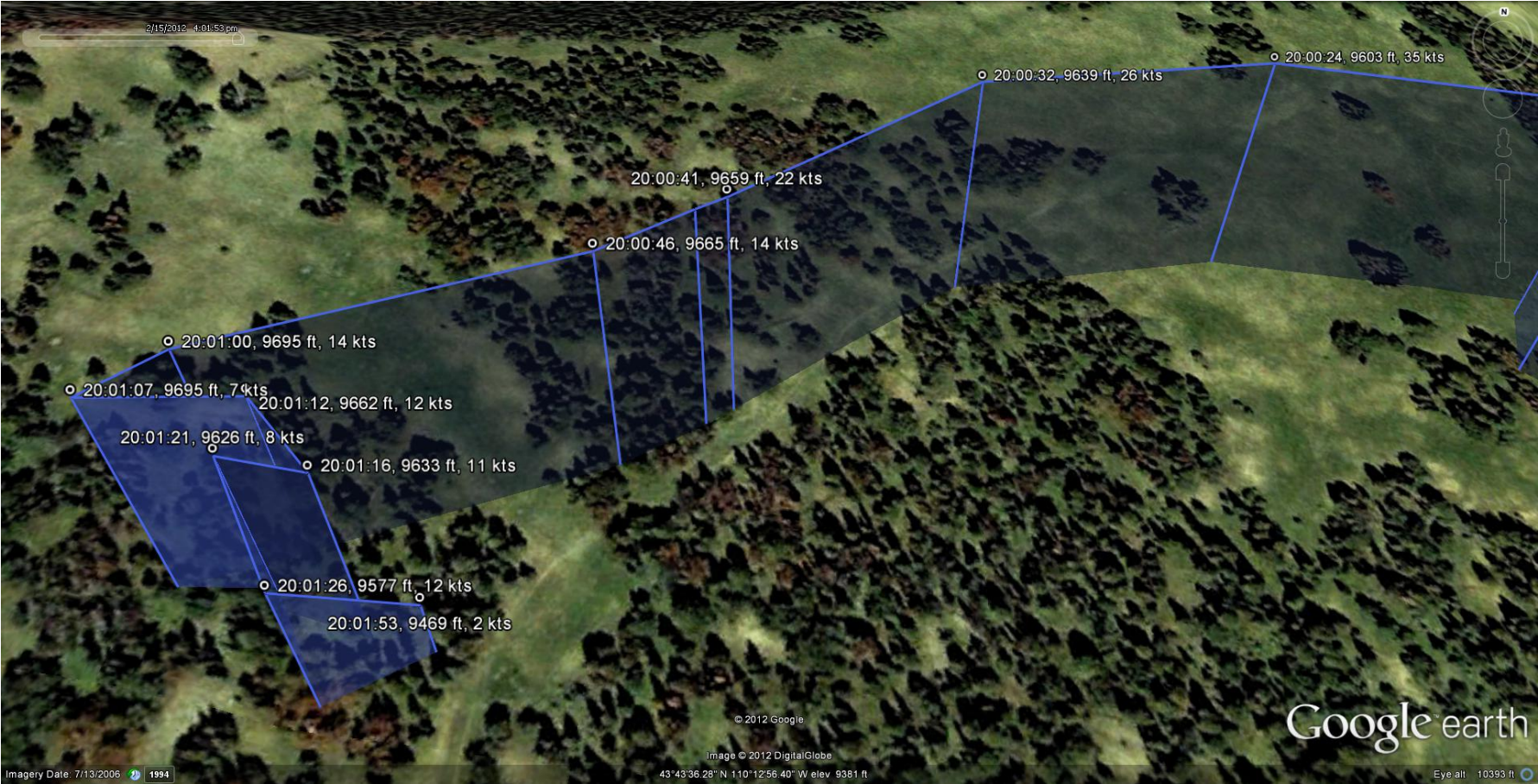
Figure 14. Last segment of flight and crash, as recorded by Garmin Aera 500.
