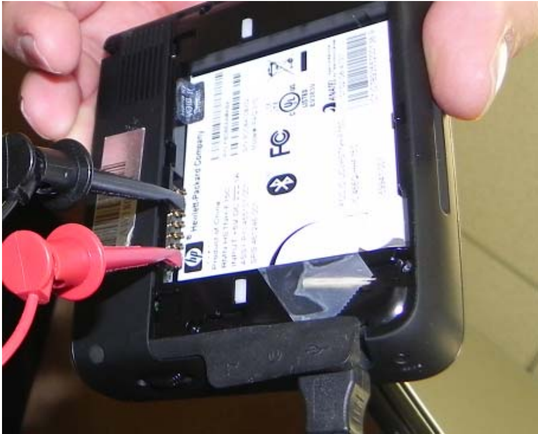
Figure 2. IPAQ connected to external power supply.
