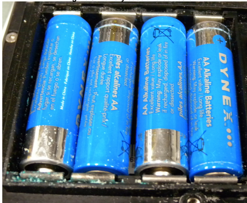
Figure 3. Battery case and corrosion.
