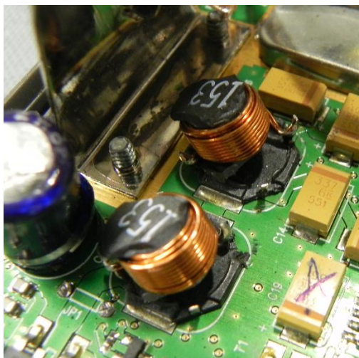
Figure 3. Photo of internal damage to Lowrance AIRMAP 2000c.
