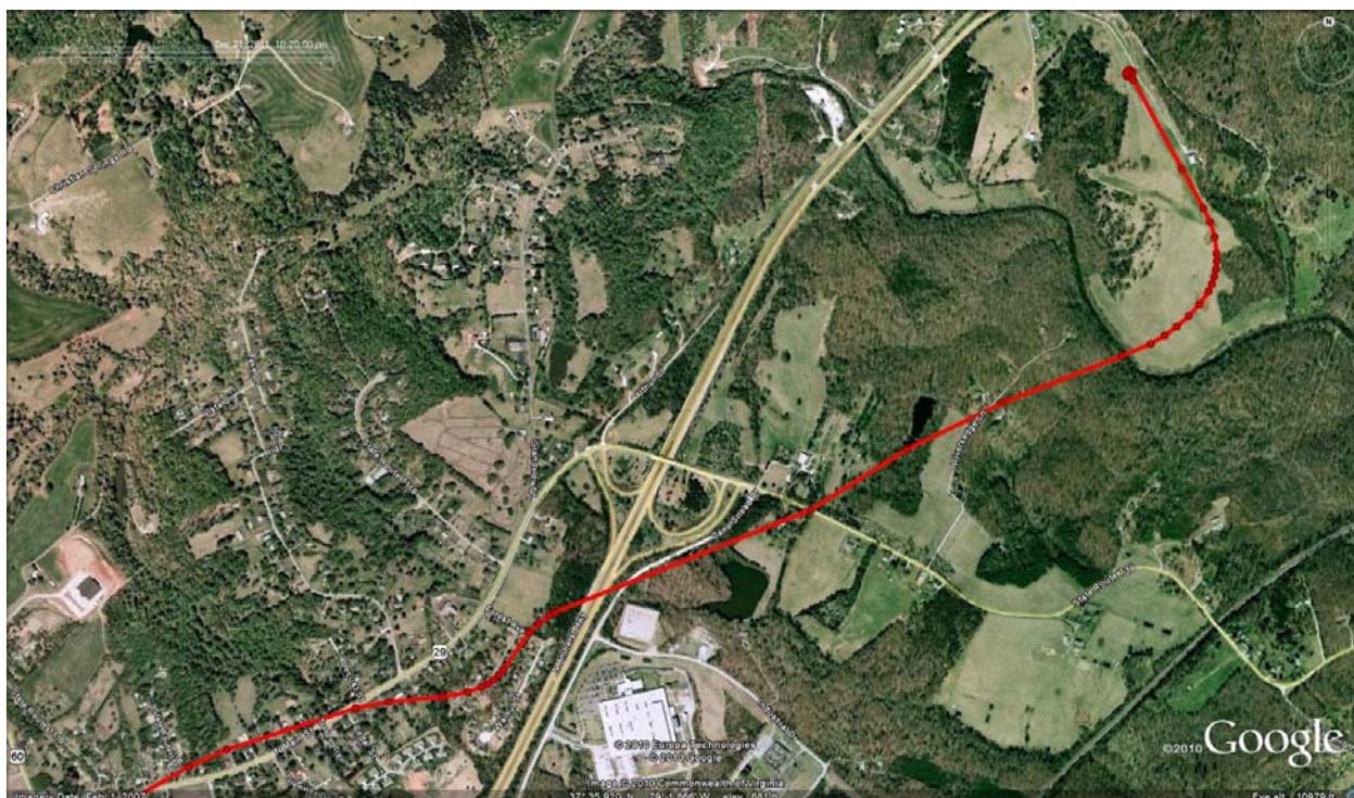
Figure 4. Google Earth overlay depicting the departure phase of the flight based on aircraft position recovered from the Lowrance Airmap 2000c (s/n 101490594).
