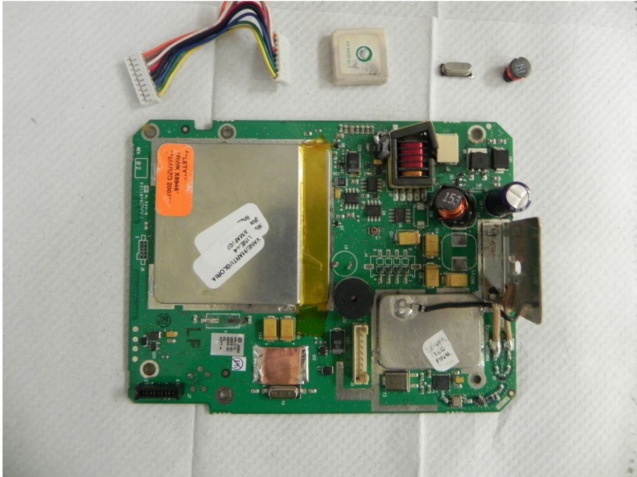
Figure 2. Internal view of the Lowrance Airmap 2000c (s/n 101490594) showing impact damage, including surface-mounted electronic parts separated from the main printed circuit board.
