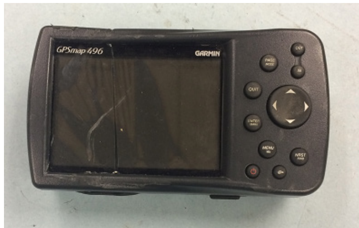
Figure 1. GPSMAP 496 with crack across display screen.
