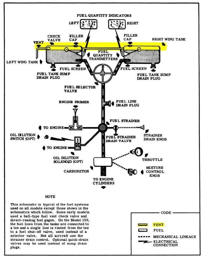
Figure 13-1. Fuel Schematic
