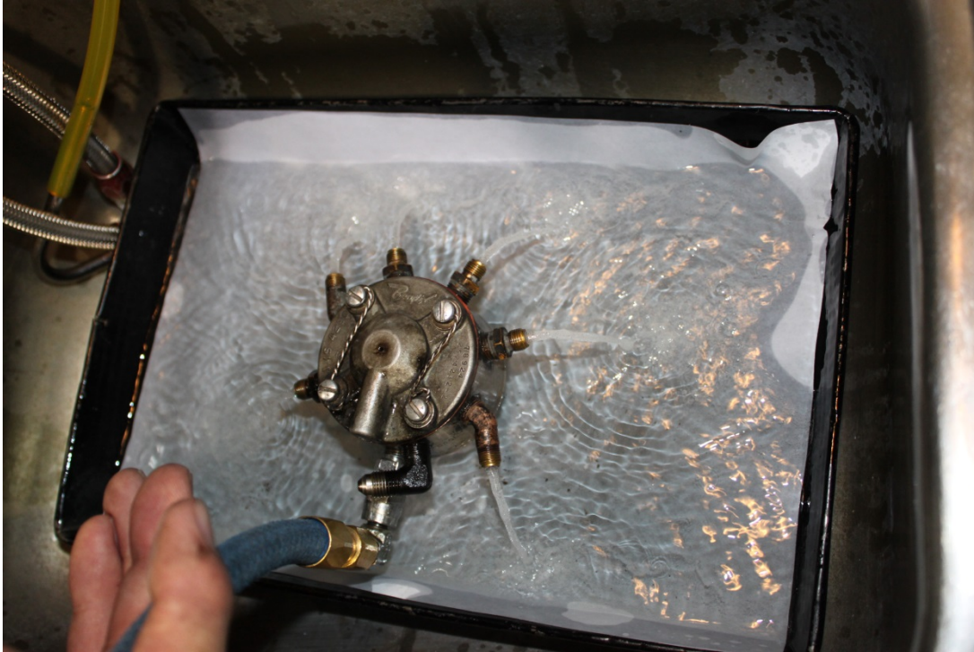
Figure 4: Bench Test at 4.5 psi of Flow Divider
