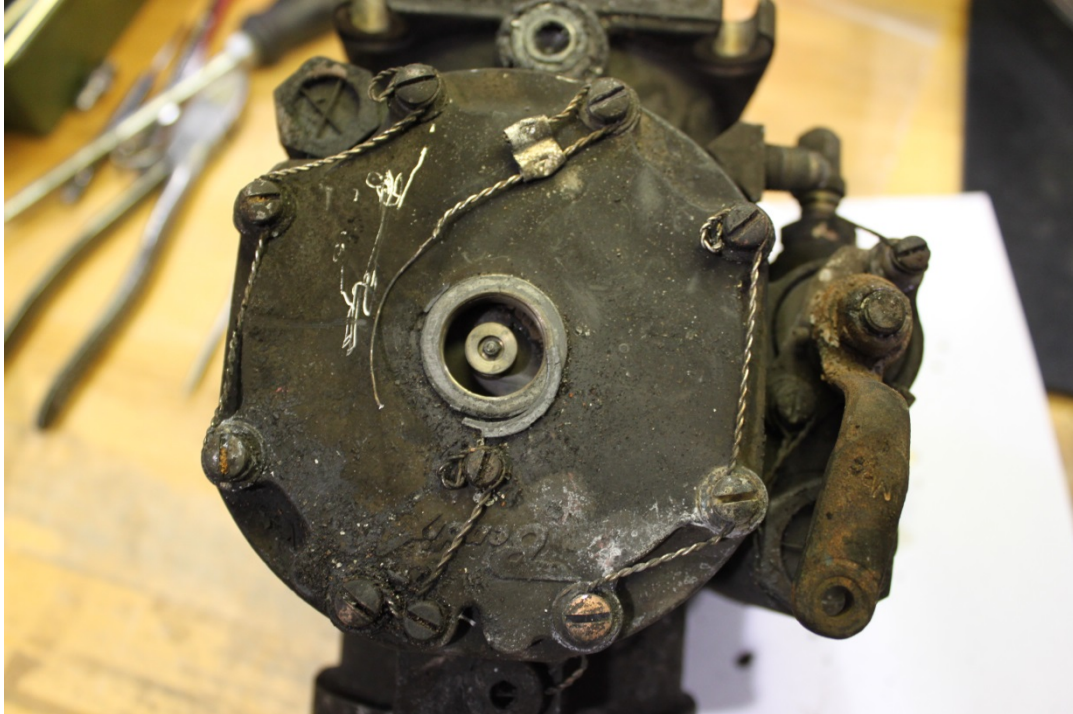
Figure 7: View of gasket material following removal of hex plug.
