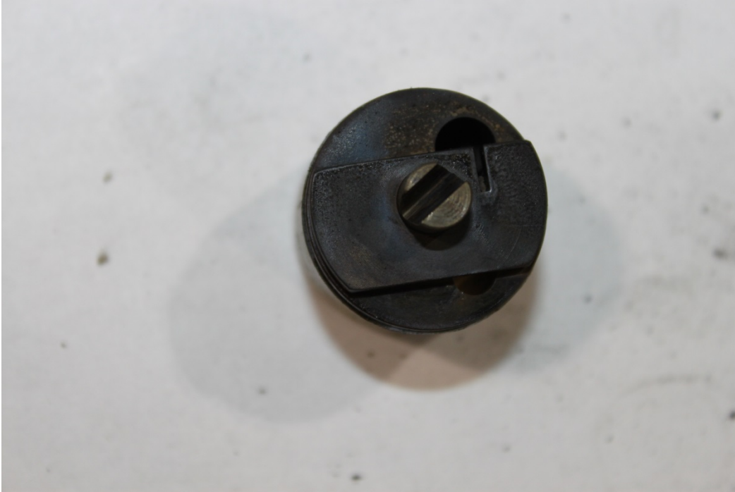
Figure 11: View showing the position of the mixture control (nearly full rich).
