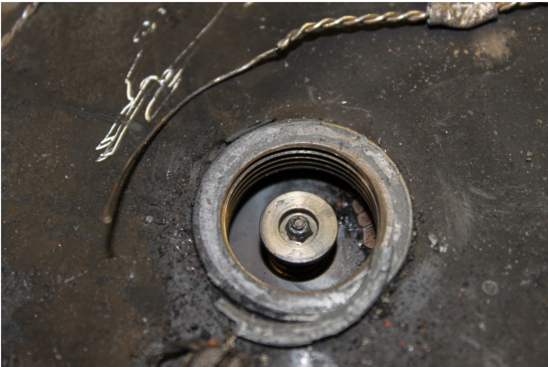
Figure 8: View showing nut installed on end of fuel diaphragm stem.
