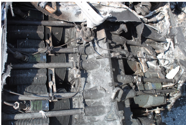
Figure 2: View of the flow divider.
