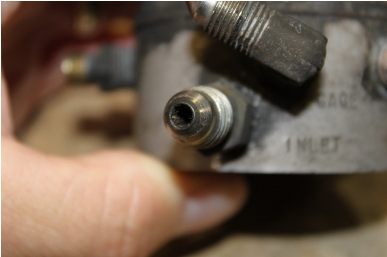
Figure 3: View of the slight debris inside the inlet fitting of the flow divider
