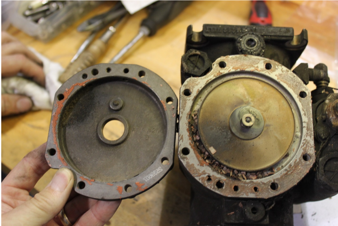
Figure 9: View of the remains of the diaphragm assembly.
