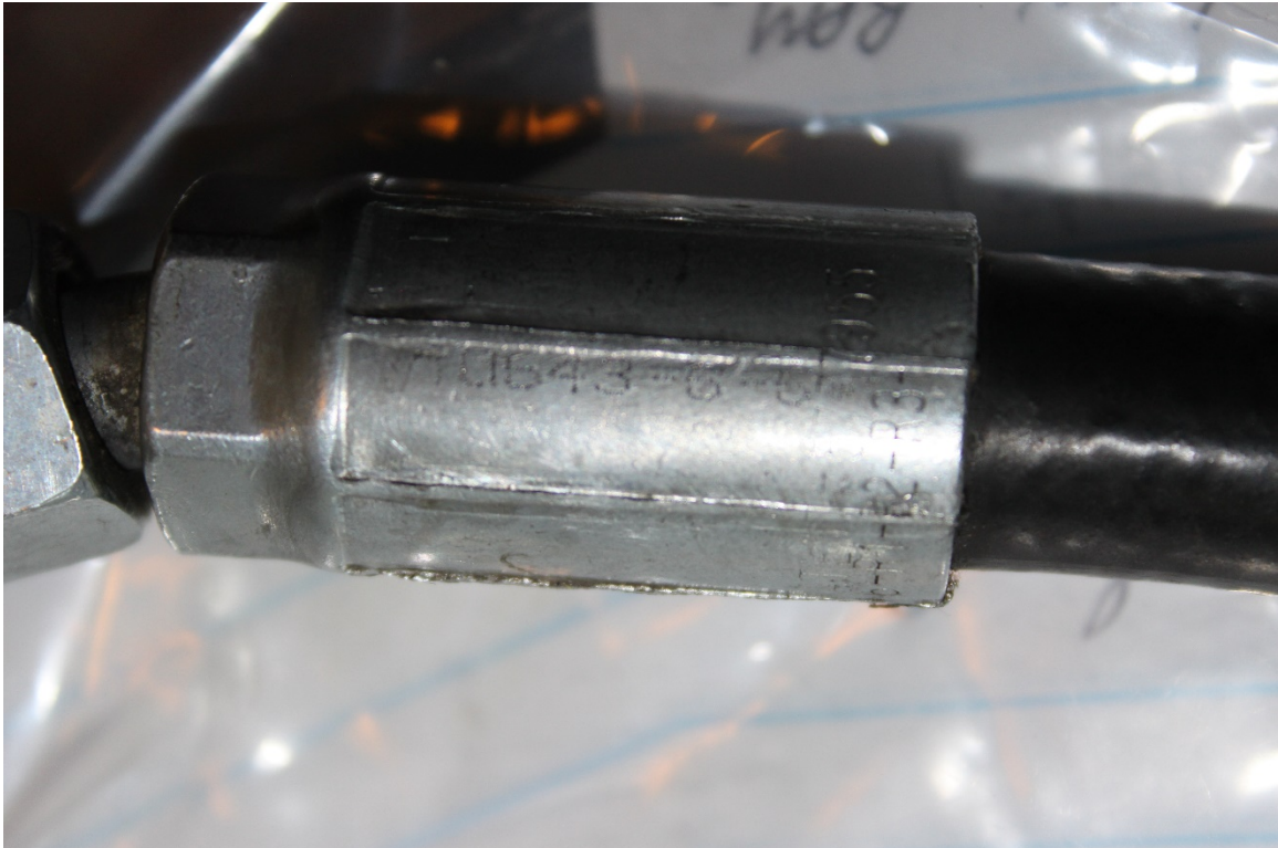
Figure 2: View of the Ferrule/Sleeve at the Outlet Hose End that Would Connect with the Fuel Injection Servo. Note the marking 10643-6-6.
