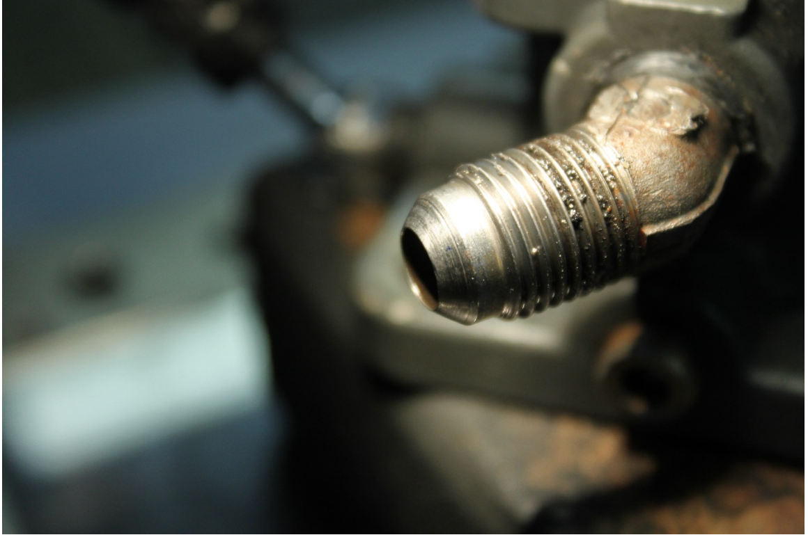
Figure 5: View of the Outlet Fitting. Note the circumferential gouge in the flare.
