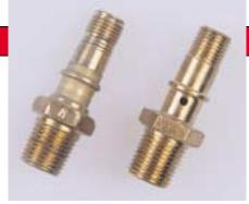
Lycoming nozzles: The nozzle on the left must be replaced due to wear caused by a loose fitting screen shroud. Always position Lycoming nozzles with the "A" facing down and the air-bleed hole up.
