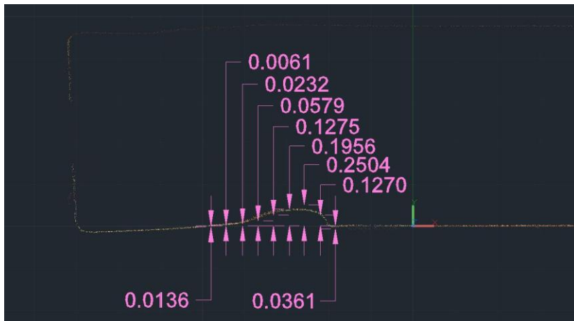
Figure 11: Crush measurements at slice A (below occupant compartment) on the accident school bus. (meters)
