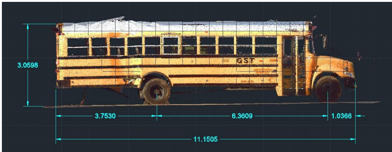
Figure 7: General dimensions of the accident school bus. (All measurements are in meters.)
