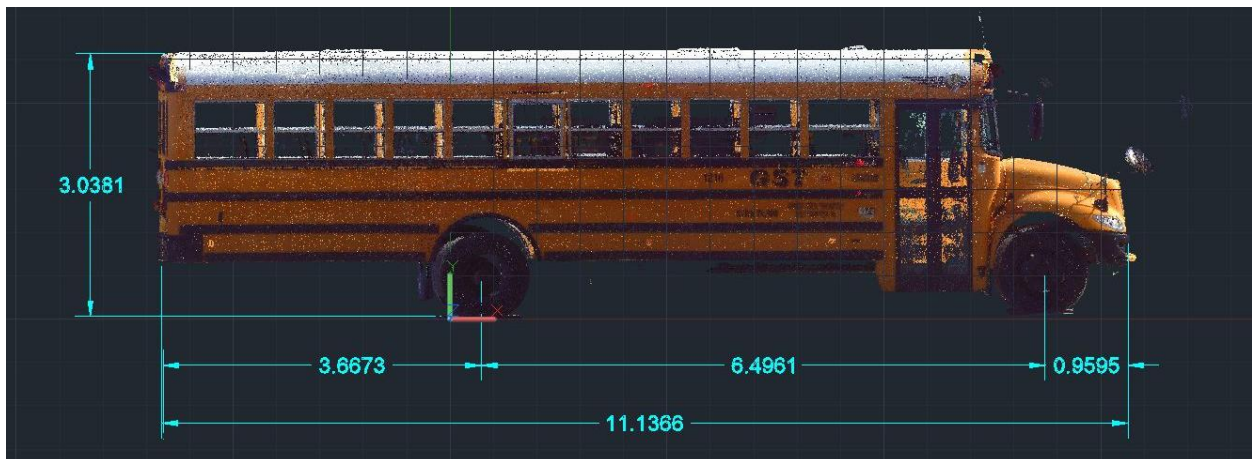
Figure 20: General dimensions of the exemplar school bus. (All measurements are in meters.)
