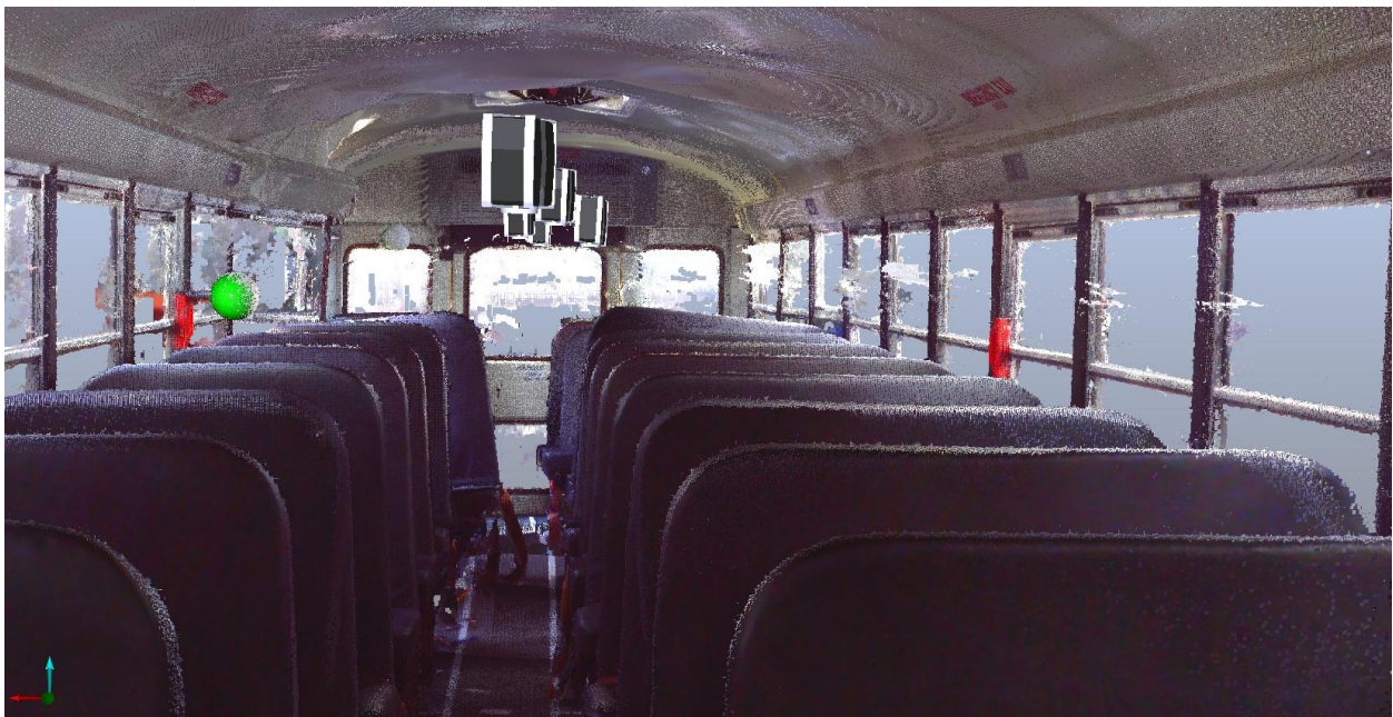
Figure 4: An image of the school bus interior from the combined 3D scan.
