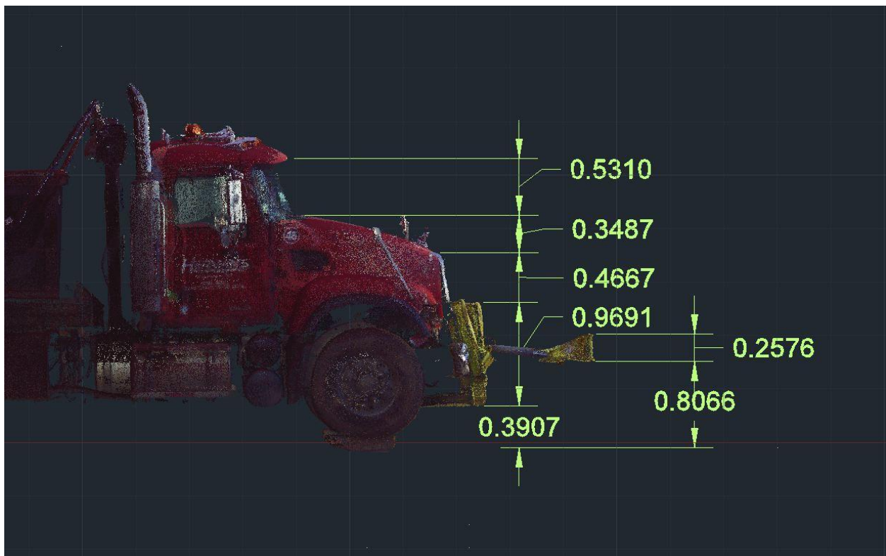
Figure 18: Dimensions of the front of the roll-off truck including the snow plow attachment. (meters)
