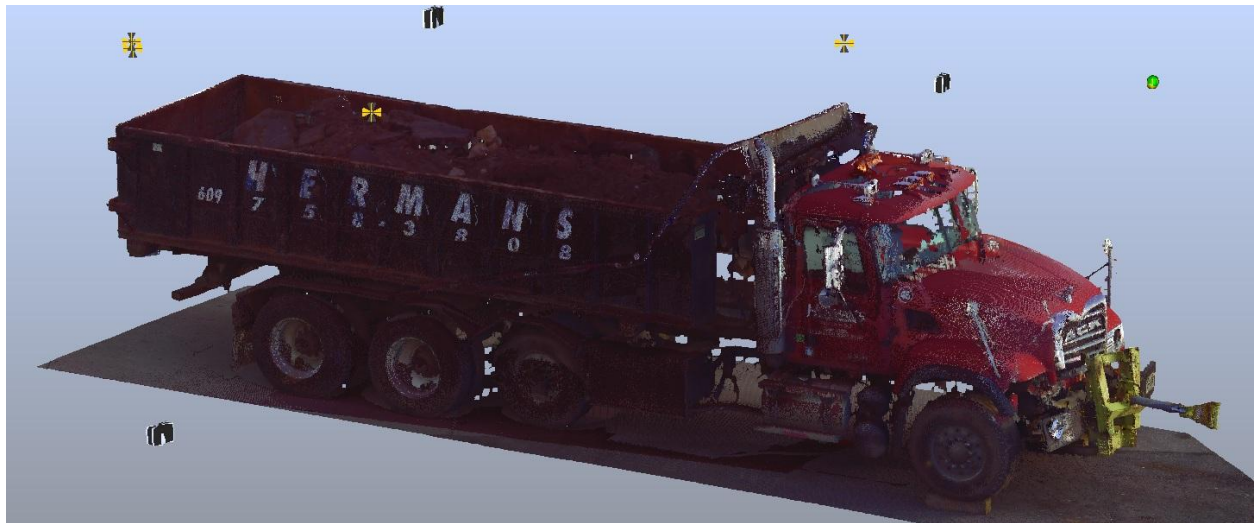
Figure 16: An image from the combined 3D scan of the accident truck.
