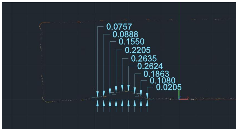
Figure 14: Crush measurements at slice D (head level) on the accident school bus. (meters)
