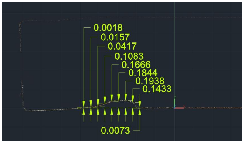
Figure 12: Crush measurements at slice B (floor level) on the accident school bus. (meters)
