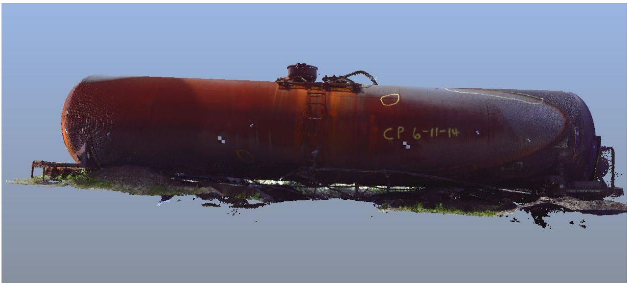
Figure 2: An image from the 3D laser scanner point cloud showing the right side of tank car CBTX 74712. The A-end of the car is shown on the left in the image. Prior to the accident the tank car was traveling B-end leading.
