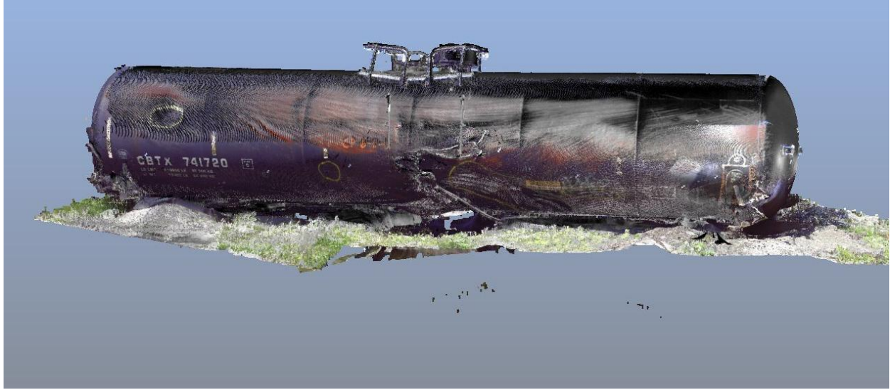
Figure 4: An image from the 3D laser scanner point cloud showing the left side of tank car CBTX 741720. The A-end of the car is shown on the right in the image. Prior to the accident the tank car was traveling B-end leading.
