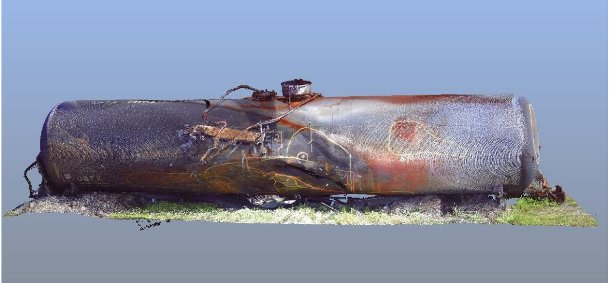
Figure 1: An image from the 3D laser scanner point cloud showing the left side of tank car CBTX 74712. The A-end of the car is shown on the right in the image. Prior to the accident the tank car was traveling B-end leading.
