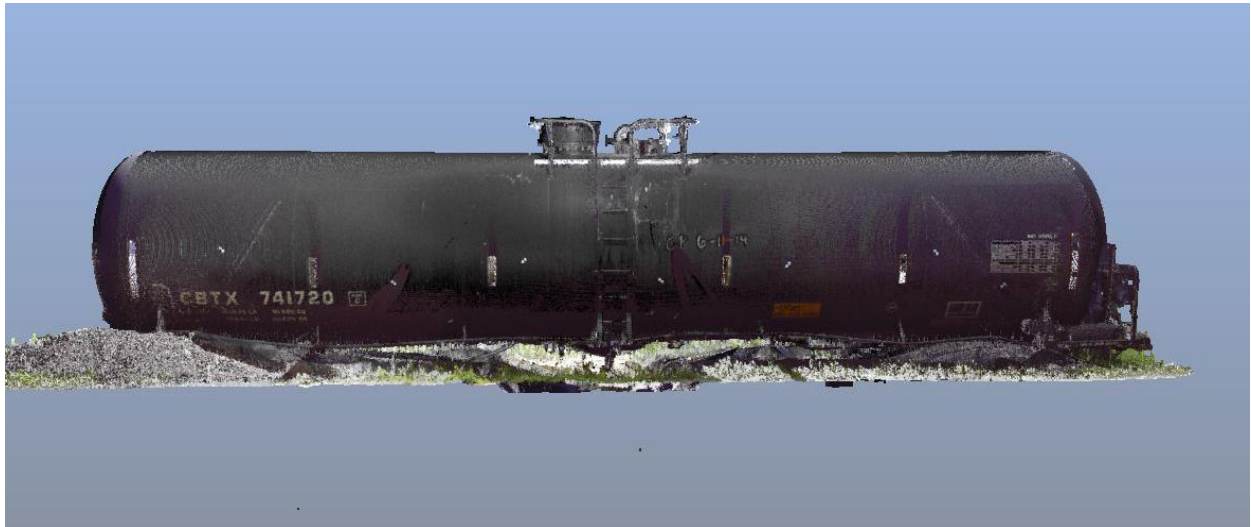
Figure 5: An image from the 3D laser scanner point cloud showing the right side of tank car CBTX 741720. The A-end of the car is shown on the left in the image. Prior to the accident the tank car was traveling B-end leading.
