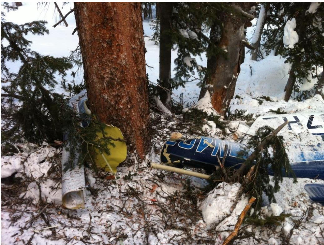
Figure 9 - Aft Fuselage and Forward Tailboom
