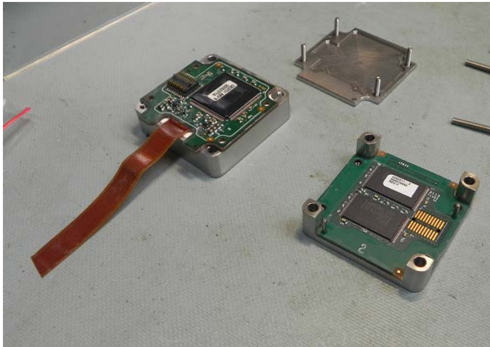
Figure 5. Component and memory board inside crash survivable memory unit.
