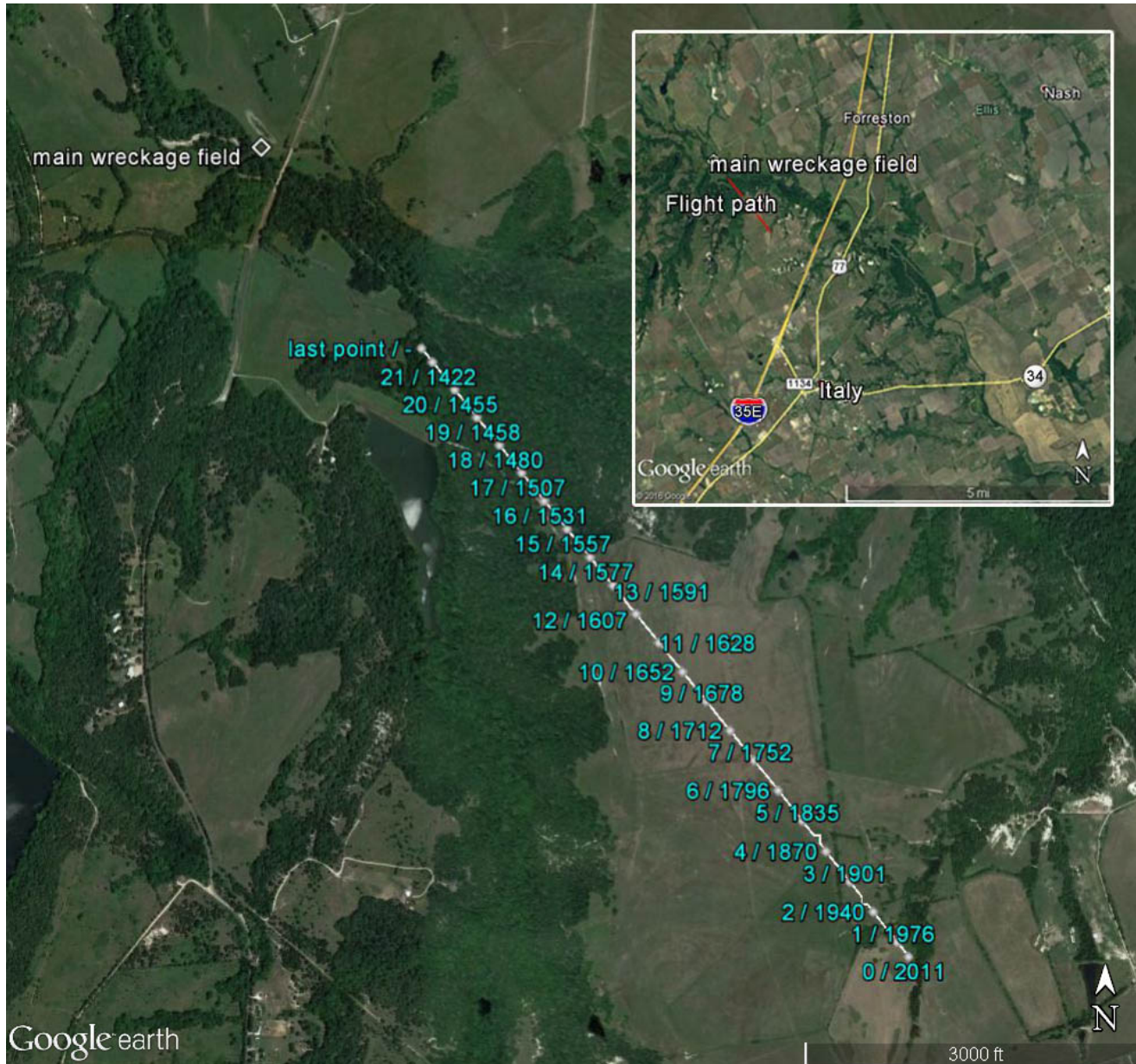
Figure 12. Map overlay of aircraft position with time and height above ground level (AGL) during test point 51.
