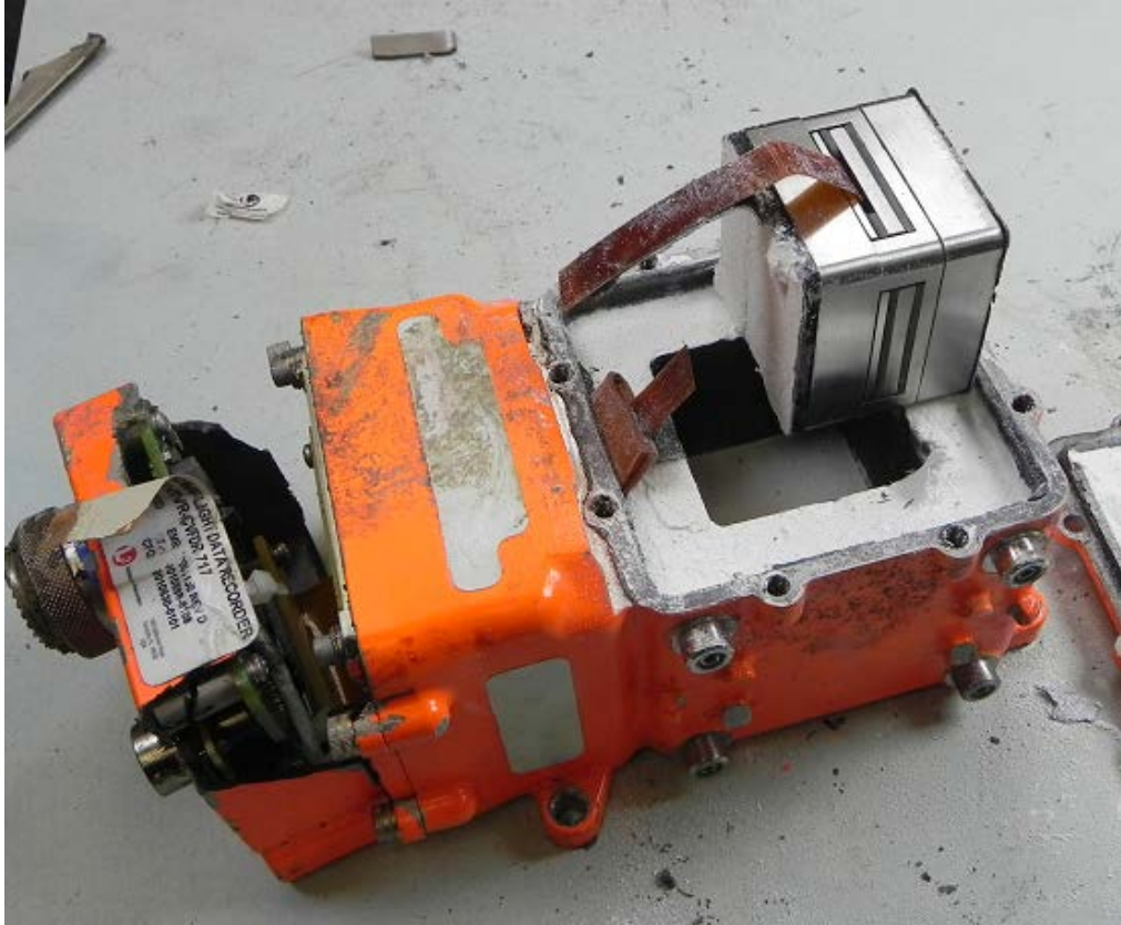
Figure 4. Crash survivable memory unit removed from unit.
