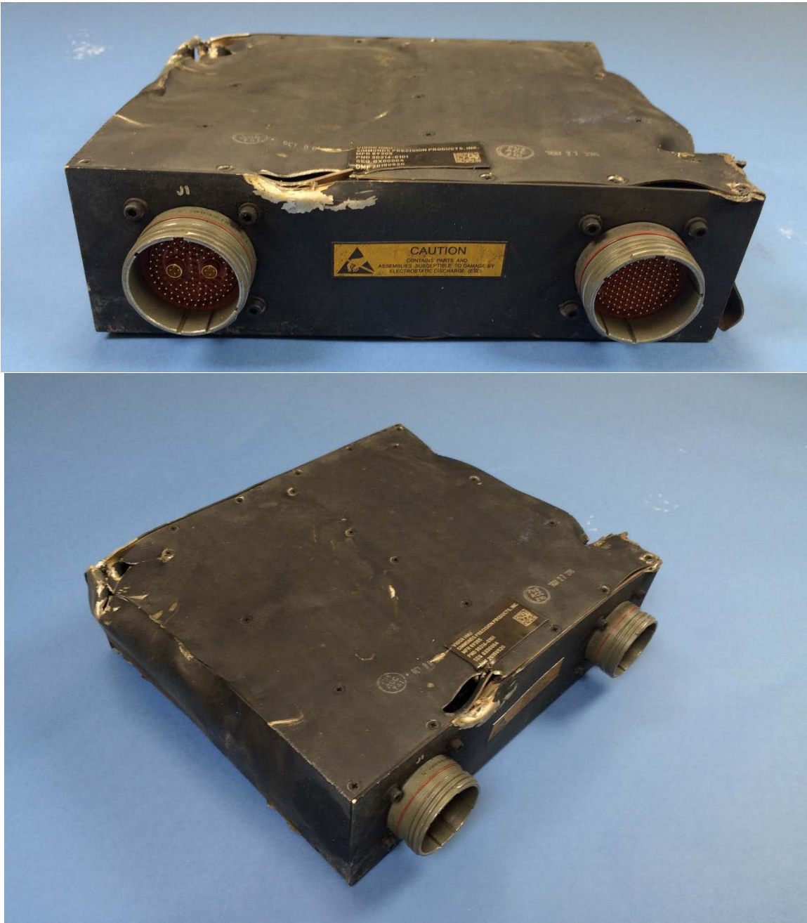
Figure 1. Exterior of Vigor HMU as-received.
