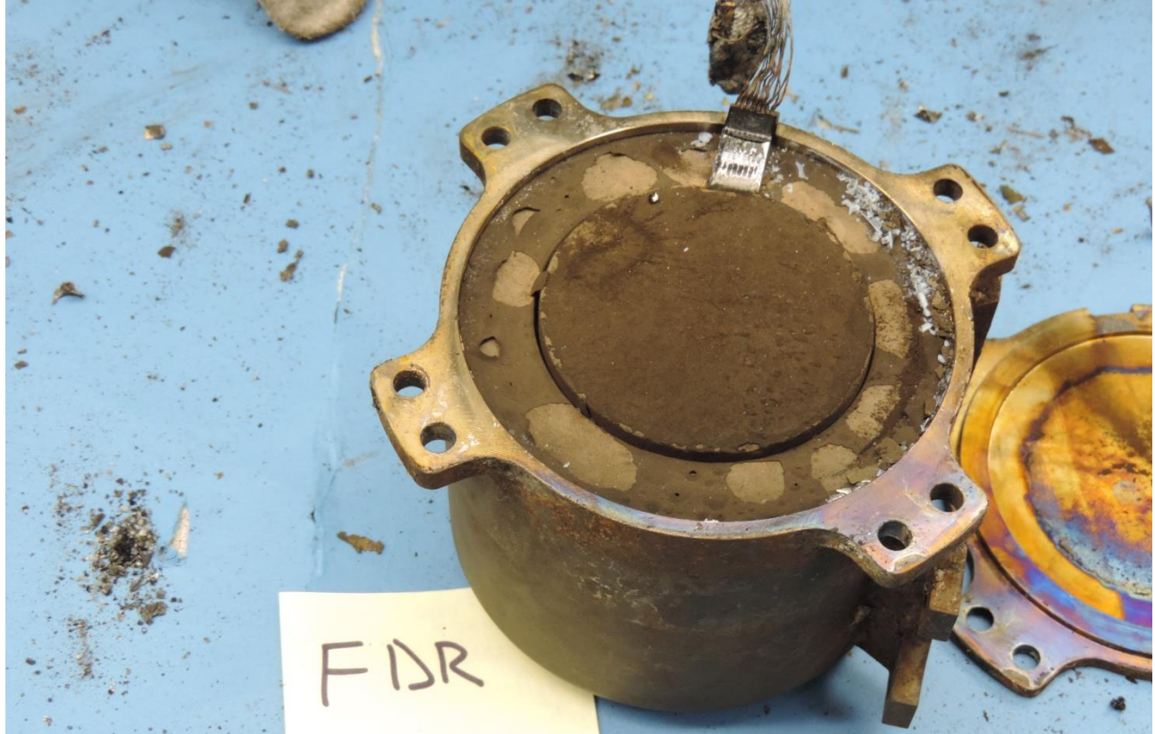
Figure 5. FDR - Crash Survivable Insulation
